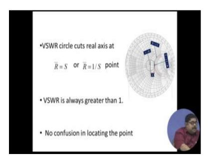
So, VSWR circle cuts real axis at r is equal to s or r bar is equal to 1 by s point VSWR is always greater than 1. So, no confusion in locating the point if you just read those 2 values of r you will understand which 1 to take. The one with higher the 1 with r value r bar value greater than 1 that will have to take the other will be always less than 1 guaranteed.
