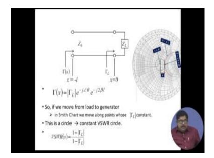
So, you see that that line reflection coefficient gamma x, I have already said that you have connected a transmission line of characteristic impedance to a load of Z l. So, there is a reflection coefficient at the load, but that is called gamma l. If you move across the transmission line your reflection coefficient value changes; that means, the ratio of voltage wave reflected wave by incident wave that changes, this is called line reflection coefficient gamma x is a line reflection coefficient.
