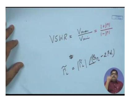
That means, when I am moving the line reflection coefficient is changing, but basically I am moving on a circle and that circle represents a constant VSWR. I say that if I move along transmission line VSWR does not change, it depends on only the load impedance and the characteristic impedance of the line.
