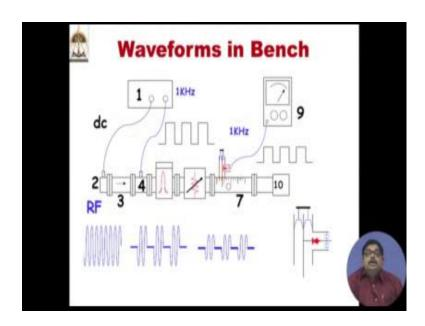
So, you have the RF thing coming from the klystron in the right, then after that after modulation that same RF waveform looks like the next one you see that, it is having some on off modulation of frequency 1 kilo hertz. So, it becomes the second waveform that is shown and then after attenuation it is like these.
