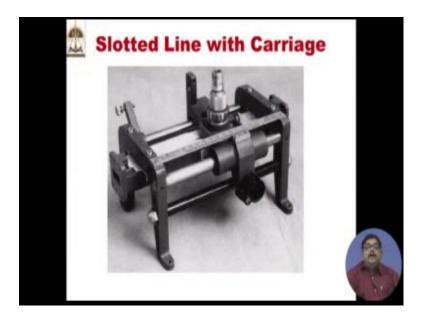
Functionally this is the slotted line with carriage this is the rectangular wave guide I was talking, you can see from the left side it is seen that this is a left side rectangular wave guide. But that probe that can move over there that is why there is a carriage. So, by that
