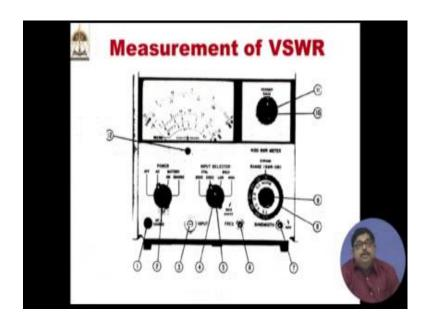
In the microwave bench we are already seen VSWR meter this is a better view of that. So, you have all used it in your labs, you will see that there are various power knobs. So, by that you can connect an AC power or external power etcetera then you can also find out the probe that you are connecting, depending on that probe, that you can get proper impedance.
