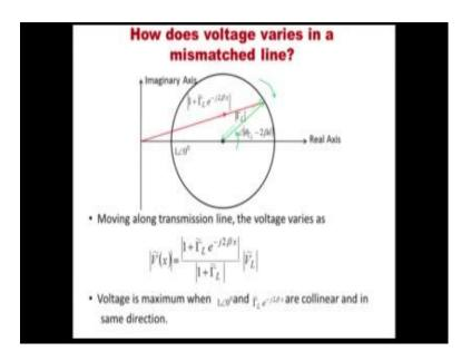
Now, these I just ask you to replace your transmission line thing, and in a trans this is transmission line stuff, that if we move along the transmission line, you can find out these that you see any good transmission line theory book and the voltage in the line voltage means this total voltage; that means, the incident voltage plus the reflected voltage that is called the total voltage.
