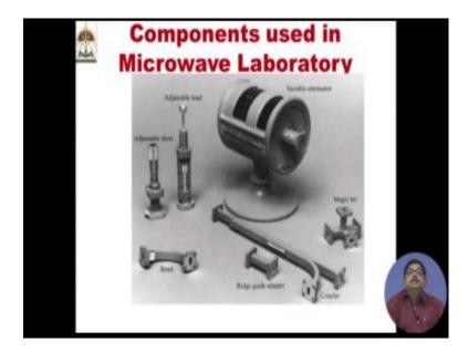
These are also required in laboratory you can see adjustable shot adjustable load, bend, ridge guide, adapter instead of power that attenuator, variable attenuator then there are two fundamental things have seen shown here one is a directional coupler; which is very
