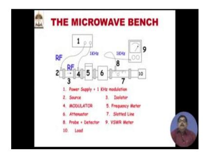
But basically if you look at that you can see these slide that same thing what we have pictorially shown. It is the same thing actually there is an RF source, but we are detecting that RF source with a diode. s I said point contact diode. So, which is on the carriage, the diode cannot detect your microwave, but it can detect a 1 kilo hertz signal.
