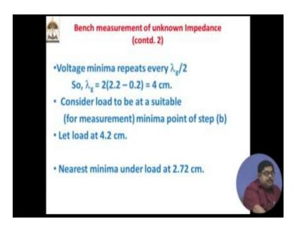
So, that is why instead of maxima we always measure the minima points. So, because it is sharply defined the voltage is at the maxima, it is flat that is why it is not, sharply defined. So, let us continue that measurement voltage minima repeat every lambda g by 2. So, we can find out by finding the difference between 2 minima position we can calculate what is the lambda g in this case it is coming out to be 4 centimeter.
