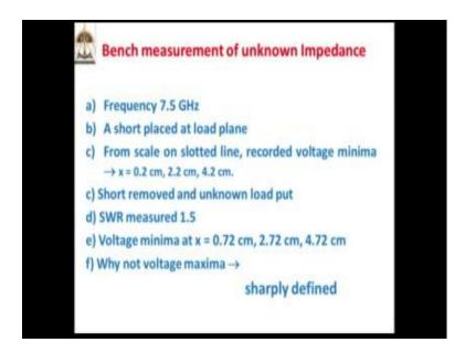
Now, typical measurement scenarios suppose frequency of operation is 7.5 Giga hertz, a short placed at load plane. Let us say we have done this experiment let us say this is recording of one of those students here measured. So, recorded when the short is placed at load plane the scale minima positions he has noted like this short removed and
