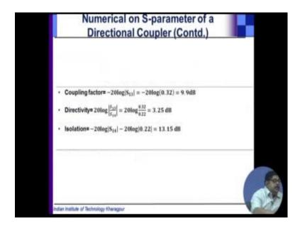
We have coupling factor, we have given the formulas in the earlier lecture that coupling factor is minus 20 log S 13. So, you can find out it is 9.9 db, directivity is 20 log S 13 by S 14. So, 3.25 db isolation see and as you can verify that in db scale. We know i is equal to b plus c. So, d is 3.25, c is 9.9. So, their sum is 13.15 and that is equal to i.
