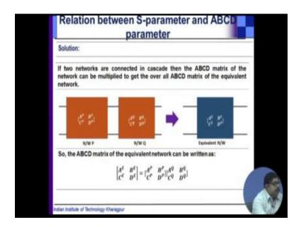
So, it is easier since this is cascade of 2 networks, we can convert to ABCD matrix and so ABCD matrix of equivalent network you know this can be written like this.
