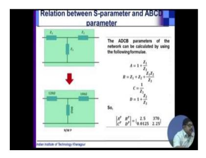
So, ABCD parameters of a tee network, you can easily find out, this is your B. Tech level knowledge then. So, the first network tee network you can find the ABCD matrix to be this, then the pie network that either you can convert to tee network and then find the ABCD matrix.
