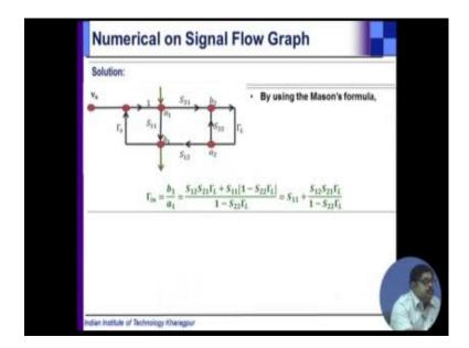
Now, the input side we have already in the lecture you can see the input reflection coefficient for a loaded 1 by signal flow graph comes to be this S 11 plus S 12, S 21 comma l by 1 minus this.
