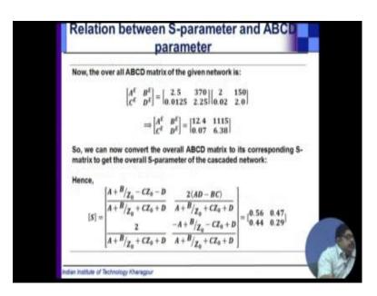
So, overall ABCD matrix is this and then this ABCD matrix can be converted to S matrix by going like that. This is to show you the usefulness of the ABCD parameter if you can convert from S to ABCD nothing like that.
