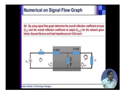
Now, the signal flow graph this problem that suppose this tee matrix was given in an earlier problem also you have also loaded thing that means, Z d L is connected Z d S is connected. So, find out the reflection coefficient and both at input and output source and load impedance is given to be 50 ohms.
