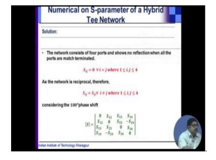
So, it is said that 4 ports and no reflection when all the ports are matched that means you can easily say that the 4 diagonal elements of the matrix will be 0 as network is reciprocal. So, you can reduce and also if you remember that 180 degree. So, 1 of the thing you can take as minus.
