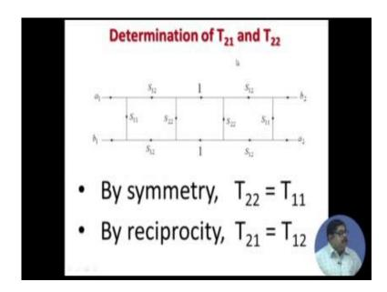
Then T 1 and T 22 you see the signal flow graph the by symmetry we can say that T 22 is equal to T 11 and by reciprocity, the whole thing is reciprocal error box is also be
