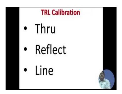
Now, TRL - T stands for Thru, Thru means a Thru line as we are showing in a direction coupler that thru line. So, Thru Reflect is line in; now what is Thru? Thru means just connecting port 1 and port 2 instead of connecting that duty if you just connect the accessible port 1 accessible port 2 of the network analyser directly together that is called Thru connection. Obviously, the male female matching will be there that is why there is some something there, but Thru.
