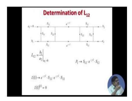
L 12, L 12 determination, L 12 is what? b 1 by a 2, b 1 by a 2, so there is direct path is there P 1 S 12 e to the power minus gamma L S 12. Is there any other path? You can go
