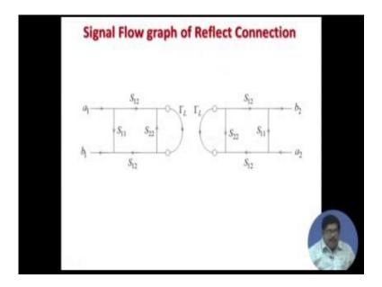
This is the signal flow graph that port 1 site, port 2 site and gamma 1 in between. So, this is the two disjoined graphs here because of the reflection connection that the port 1 that is getting fully on its own similarly port 2 is getting on its own.
