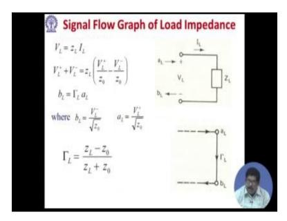
Similarly, signal flow graph of load impedance is load, there is one incident, one reflected wave; so, their relationship is a load reflection coefficient.
