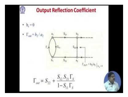
Similarly, you can find it out from output reflection coefficient; that output reflection coefficient will be this b 2 by a 2. That means how you can come from a 2 to b 2? So, there are, again, if you put that, that one path is this; another path is, go here, come here; so, then find out, what is the loop; there are, one loop is here; another loop is, you can say that, this is another loop. So, these two loops, you do that, and you can get this.
