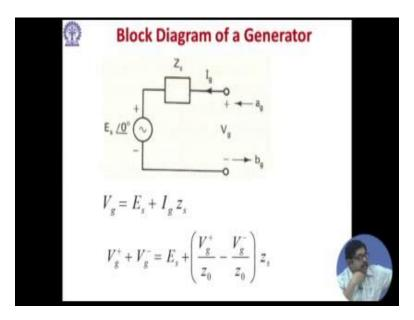
Similarly, you see a block diagram of a generator. So, we know that, V g, the total voltage that is open circuit voltage you are getting, that will be E s plus I g into z s. Now, V g, you can break into again two parts, that V g plus and V g minus; V g plus you call a g, and V g minus you call b g; so that, again is written here.
