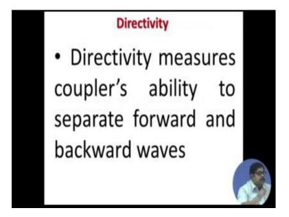
Now, directivity measures couplers ability to separate forward and backward waves. As I said that if you go back to this diagram that you see in this second one, it is showing that directivity means how much I am going here and how much here. Now this is incident wave, incident wave is going to port 3 and whatever is reflected at port 2 that is coming here as port 4 and they are getting separated. Till now we have not mentioned this point,
