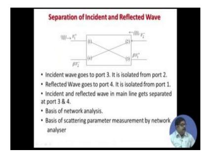
Now, separation of incident and reflected wave, as I said incident wave goes to port 3 it is isolated from port 2. Reflected wave goes to port 4, it is isolated from port 1 incident and reflected wave in main line gets separated at port 3 and 4. This is the basis of network analysis, basis of scattering parameter measurement by network analyzer. So, that is why it is so important to understand directional coupler.
