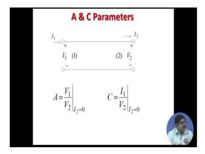
So, this is the definition now to find in A, B, A and C you see in both these cases we require I 2 should be made equal to 0. Now, I two; that means, if we make in the port 2 I
