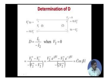
And determination of D that is ratio of 2 currents this, so that will give you this D is equal to cos beta l and again a real quantity.
