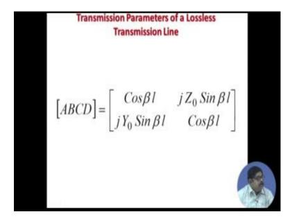
So, finally, you get the transmission parameters of a lossless transmission line to be cos beta l j Z naught sine beta l etcetera.
