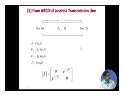
So, if we put that then we have ABCD we have written A once again here, if you do those conversion formula you get that S parameter of the lossless transmission line is its S 11 is 0 its S 22 is also 0 its S 12 and S 21 are e to the power minus j beta 1. So, as you see that this S parameter from the S matrix we can see it is a reciprocal network because there are no active devices etcetera is used. So, its S parameter is reciprocal; that means,
