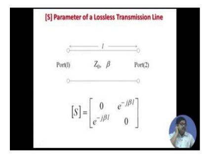
So, now you know that if you have any circuit, if it is distributed circuit it is better to find its S parameter because actual transmission is happening through waves. So, you can find S parameter then S 2 Z you can reconvert back that formula is given here.
