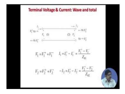
So, you see we have a piece of transmission line of length 1 characteristic impedance of the transmission line is Z naught phase constant is beta that means, we are assuming lossless transmission line. So, propagation constant gamma that does not have any real part, it has the imaginary part j b that is why the face constant is only shown.
