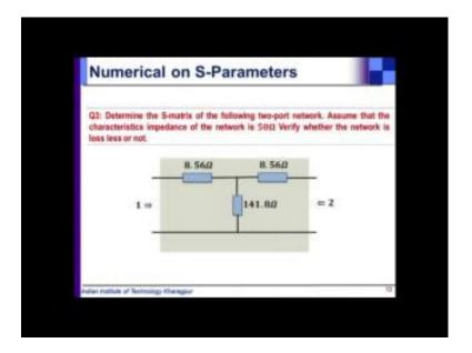
In c1 port is shorted, other port return loss. Now see the third problem, that S matrix of the following 2 port network. Again verify whether the network is lossless or not, that you see this is a purely lumped element case.
