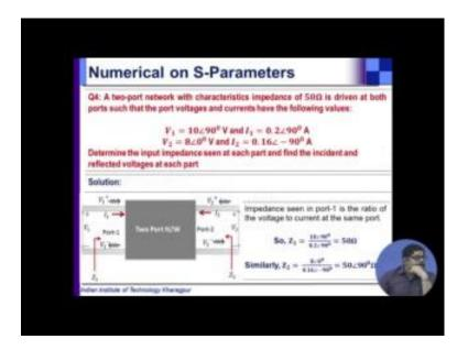
Now, it 2 port network with characteristic impedance 50 ohm is given at both ports, such that these are the various port voltage and current values. So, determine the input impedance seen at each port and find the incident and reflected voltages at each port. So, it is given at both ports. So, impedance seen in port 1, self impedance that will be a ratio
