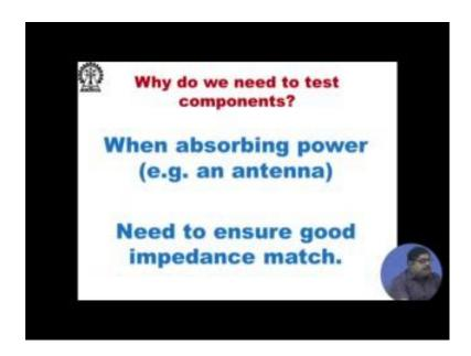
Also suppose we are giving power to an antenna. Now, we need to ensure good impedance match whether whatever power we are supplying to the antenna whether antenna is radiating there.
