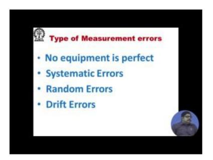
No equipment is perfect, it has some systematic errors, some random errors, some drift errors, systematic errors means suppose I am saying that it should be defined, I want a perfect impedance match, but in reality I cannot always get impedance matched I say that at the port the terminal should be defined. In actual reality the may be port is extended a bit.
