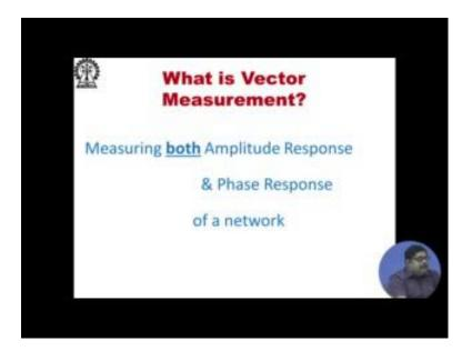
Now, what is vector measurement measuring both amplitude response and phase response of a network is called vector measurement. Network analyzers are available who does scalar, who are called scalar network analyzer they do not measure phase response they measure only amplitude response.
