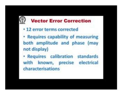
Now, vector error correction they are if you do this model 12 error terms are corrected, requires capability of measuring both amplitude and phase, requires calibration standards with known precise electrical characterization.
