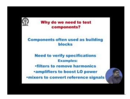
Now, why do we need to test components at microwave components often used as building block microwave frequencies. Now, we need to verify specifications like filters, we need to see how much harmonics it is removing amplifiers whether the local amplifier power is local oscillator power is sufficient or not mixers whether it is properly rejecting various signals.
