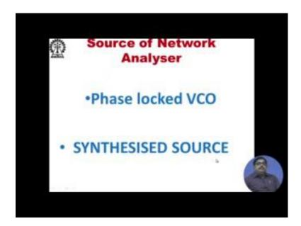
It processes and displays, now source of network analyzer it either a phase locked VCO; voltage control oscillator or a synthesized source synthesized source means the source at a particular frequency then from that various into 2 divide by 2 etcetera. So, that the source was having a particular range from that it synthesizes some other ranges. So, the source becomes a broadband source and gives lot of frequencies.
