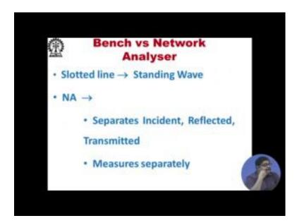
Now, network analyzer it is predator was microwave benches. We have seen microwave benches in the impedance measurement time, basically they work on standing wave network analyzers, do not work on standing wave phenomena they can separate incident reflected and transmitted wave.
