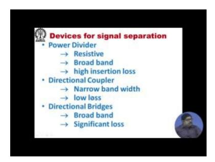
Then it takes a reference and it makes a ratio measurement. Now, if you make ratio of any measurement then your error becomes less devices for signal separation. I earlier said directional coupler along with that you can also have power dividers, but it has high insertion loss. Directional coupler is a very good it has narrow bandwidth low loss also directional bridges are used, but out of this directional coupler is one of the popular device for signal separation.
