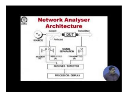
This is the network analyzer architecture it is having source is producing incident thing, then the thing is given DUT is the network that you are trying to test. So, it is giving reflected. Now, it can separate these incidents and reflected as you see here that. So, that goes to two parts incident and reflected and then also it samples the transmitted one. So, these 3 is given 2 various, 3 or 4 number of detectors and then.
