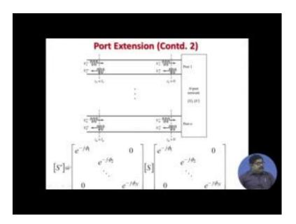
S parameter that will be even by this that port 1 is extended by let us say or theta. Now, we are calling phi, phi 1 then port 2 by phi two, etcetera. So, you write the matrix like
