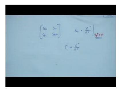
We have S 11, S 12, S 21, S 22 and what is S 11, S 11 is V 1 minus by V 1 plus when V 2 plus is made 0 match load, now is S 11 equal to deflection coefficient in general what is
