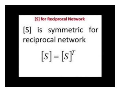
Now, various times we see that a network is reciprocal then if we do not use any non reciprocal device, 1 of the very popular non reciprocal device is ferrite. So, if ferrite is not used or other such non reciprocal special materials not used, in most of the passive devices they are symmetric or their reciprocal network.
