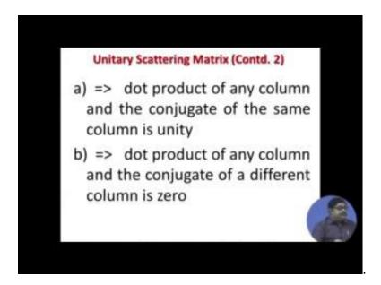
So, that we are saying the dot product of any column and the conjugate of the same column is unity dot product of any column and the conjugate of a different column is 0. So, both the things should be simultaneously satisfied, if any of them is highlighted it is not unitary scattering matrix that means, the network is not lossless.
