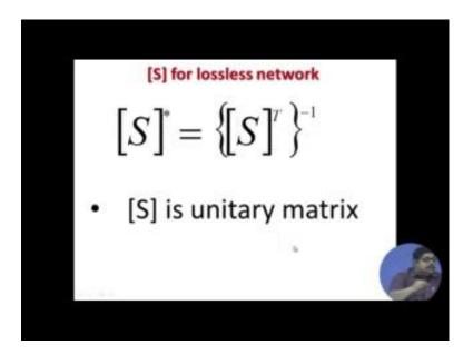
Now, if a network is lossless, lossless means there is no dissipation of power, there what about is in studying inside, there is no loss that is called the lossless network. So, for a lossless network, the S matrix is this property you see S conjugate is equal to S transpose inverse that, now, if you remember any network whose conjugate is equal to inverse of transpose that is called a unitary matrix. So, for a lossless network, S is unitary matrix.
