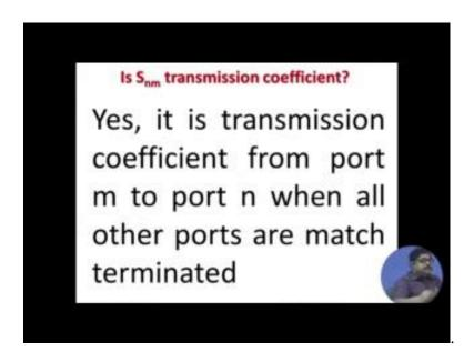
Is S n m is transmission coefficient again our answer is yes or no. So, it will be yes when it is transmission coefficient from port m to port n when all other ports are match terminated. So, this match transmission is important other ports match terminated then is parameter S and m are transmission coefficient. So, in a 2 port network say that easiest one.
