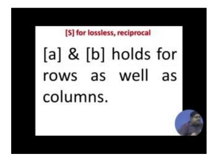
So, if any you have resistance used in the network you can see that is S matrix cannot be lossless a and b holds. So, now, if lossless as well as reciprocal material network that case the property holds for rows as well as column because for reciprocal the network and its transpose is same you know columns after transposition becomes rows.
