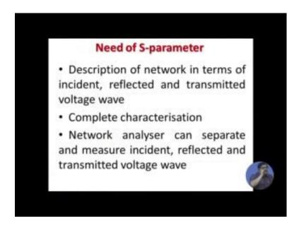
Z Y h, a, b, c, d we still can do indirectly, but if you want to measure this parameters then we need to measure the separate wave quantities and that is why there was need to define a new 2 port parameter that is called scattering parameters.
