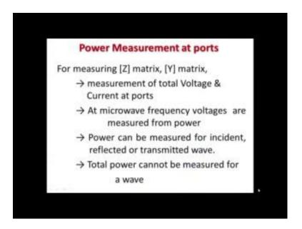
The second tool, we know that at ports we do power measurement because at high frequency is very much necessary that exactly at ports, we need to define powers because at other points the power measurement will be different. Now, for measuring that at 2 port network or any import network, linear network it characterize by Z matrix or Y matrix and for finding Z matrix or Y matrix of an network, we need to terminate properly the ports and measure either voltage and currents.
