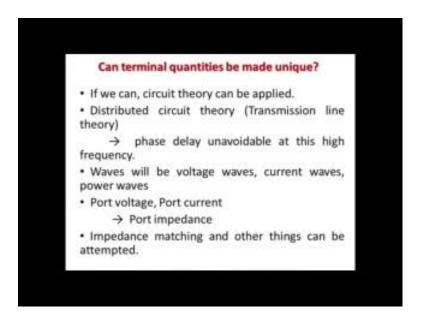
So, the question is can this terminal quantities been made unique now obviously, phase delay is unavailable at this high frequency as I said that here, since we are very high end of frequency gigahertz sort of frequency or several megahertz of frequency several hundreds of megahertz of frequency. So, even a small length that adds to quite good amount of phase. So, we cannot avoid the phase delay.
