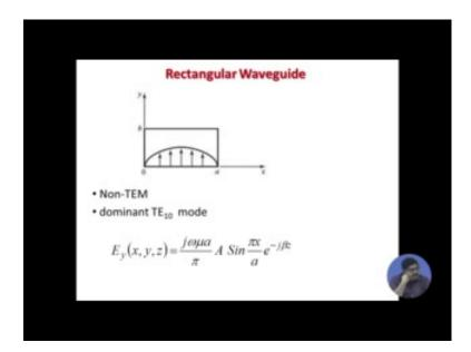
But, let us see rectangular waveguide, rectangular waveguide as dominant field distribution as TE 10 it is a non TEM mode and electric field. The transverse electric field it has only 1 transverse electric field it is along the narrow dimension of the waveguide that is generally we call y e direction the expression is given the variation is along x the variation is shown in the figure and it is a sinusoidal variation the wave is propagating in the positive Z direction.
