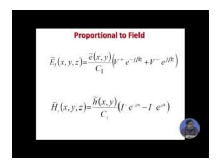
Now, see that the guidelines for defining equivalent voltage current the 2 first points are the equivalent voltage is proportional to the electric transverse electric field that is why we are writing e t x, y, z that should be written as V plus y c 1, c 1 is constant obviously, the eigenfunction will be there, but other parts we are writing as V plus by c 1. Similarly, the magnetic field is meant made proportional to the current the constant of proportionality in this case is c 2.
