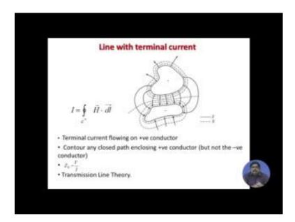
Similarly, we know that the closed line integral of magnetic field gives us current. So, here the terminal current that is flowing on positive conductor, if we can have that current uniquely defined for any contour closed path enclosing positive conductor then we can define the ratio of voltage and current. So, defined as the impedance and this is basically the realm of transmission line theory.
