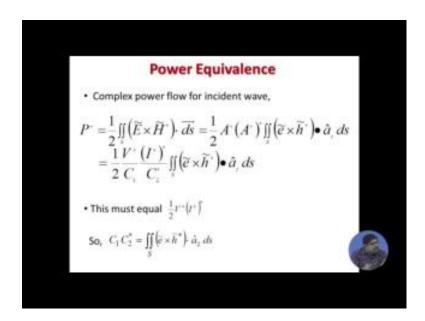
Now, we are forcing the power flow condition that instantaneous power flow should be the product of voltage and current. So, if we assume time harmonic fields, that is sinusoidal fields are one form of time harmonic field e to the power j omega t, then we can also define an average power wave power flow.
