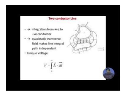
So, first let us see a 2 conductor transmission line which is the quasi line when it is extended up to gigahertz in up to gigahertz, nowadays it went to 10-20 gigahertz, it is huge, it is modified a very good designed quasi line nowadays can work up to 20 gigahertz also and this in this picture you are seeing that if we have 2 conductors 1 is positively charged another is negatively charged and obviously, there will be electric fields and magnetic fields between them.
