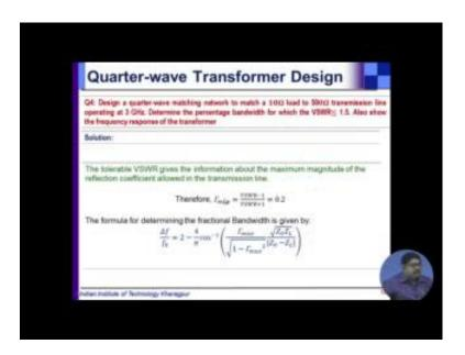
You can plot the frequency response also. Now, then design a quarter wave matching network to match a 10 ohm load to 50 ohm transmission line. So, here you see that if you
