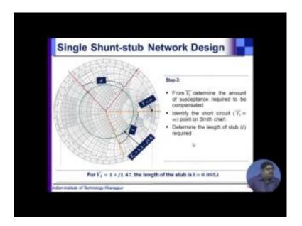
Then determine the amount of susceptance so you read this value and find out, suppose here Y 1 is equal to 1 plus j 1.47; that means, now I will have to have the shunt stub and I want that stub should then balance this class j 1.47; that means, shunt susceptance will be minus j 1.47.
