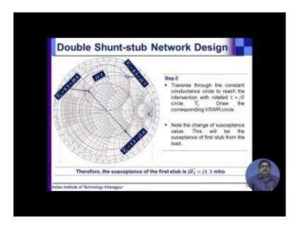
Then, traverse to the constant conductance is the load Y L, now traversed to the constant conductance circle to reach this circle. So, that is this part and you are reaching here. So, this is one solution you can continue and you can cut this in another point also here; that means, if you continue it here come, here another solution will be here.
