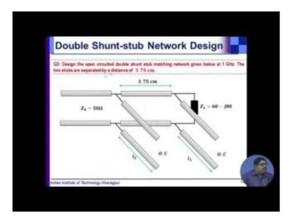
Similarly, double shunt stub matching network, you see this single stub that has a frequency response and you can plot it like this.
