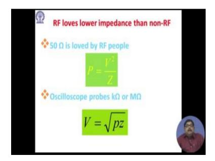
Now, another thing is you see, generally since the same reason that we are scarce of power. So, RF at RF people they the instruments, etcetera that is designed generally for 50 ohm of power 50 ohm of 50 ohm impedance. So, it is a small impedance whereas, oscilloscope probes they are kilo ohm or mega ohms sort of impedance you have seen that in your oscilloscopes the probes that are coming there you can change it to 1 ohm or 10 ohm probes etcetera.
