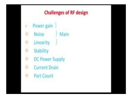
Now, what are the challenges of RF design briefly that we need to consider various parameters you see, one of the parameter is power gain not voltage gain. The next is how much noise because since you are opening up to the outside world, you are also giving or taking lot of outside noises, suppose a lightening takes place, suppose some star is radiating radio star all those your antenna is picking up. So, you are getting noise.
