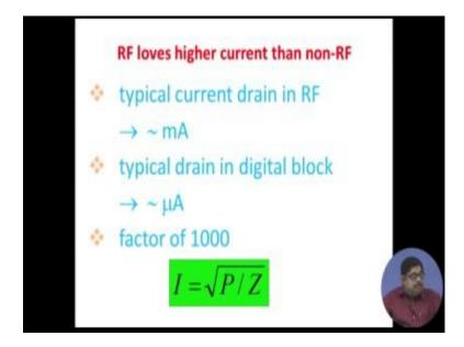
Then also typically the RF has higher current drain, typically of the order of milli ampere whereas, in a typical digital block particularly with semi-conductor technology you have of the order of micro ampere or even smaller. So, current wise RF people they have more power compared to that again due to the same reason that the impedance is small. For RF people, that is why the current for the same power the current will be higher in case of RF designers.
