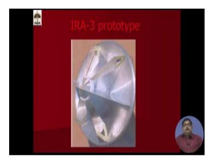
This is a better view of that antenna and you can see it is a dish antenna, but there are serve on the back of it, there are transmission lines properly designed. So, that a pure pulse almost an impulse sort of thing you can radiate to them.
