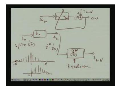
It take the receive signal R n, it constructs an adaptive filter, because this equalizer is a causal if I get system of length 2 n as I shown. So, you construct and equalizer here, may be from w 0 dot dot dot w 2 N minus 1. This output should be as close as possible to got not In, but In minus n. In is 1 that transmitted sequence, that pilot sequence, it has delayed by N because; you know that your channel could have been, I mean this equalizer actually is non causal, but you have merit causal.
