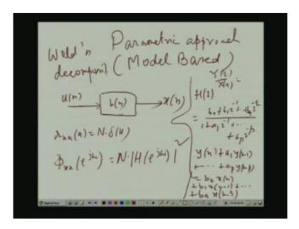
Model based here the entire problem of estimation of the power spectral density can be made to boil down to an equivalent problem of estimating estimation of a few parameters for the model. And very sophisticate algorithms exist in literature. Now, before I going into that just consider this view. That suppose there is a lti system linear shift and linear system of impulse response hn. It is excited by a white process un 0 been white process output is xn.
