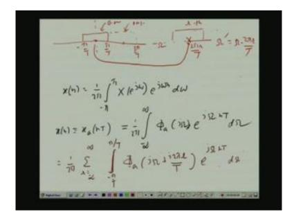
This is my origin. So, I will have 1 slot or 1 sector from minus phi by T to phi by T this I call it zeroth. Then phi by T to 3 phi by T dot dot dot dot r th will be where. If you for zeroth means the sector is from minus phi by 2 to minus phi by T center is 0. Then the first 1 first is here here the center is at 2 phi by T. And we go phi by from 2 phi by T we go phi by T to the right and phi by T to the left to go to meet to boundaries this.
