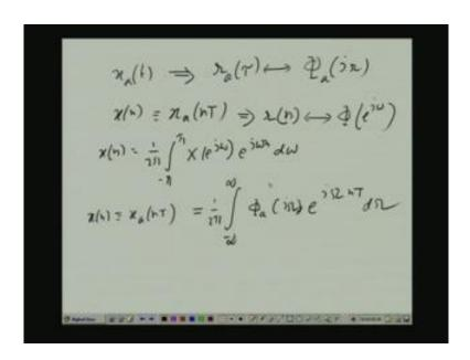
That is suppose there is a random continuous value that is analog random process xa t. And this is sampled at a time period sampling period of T to generate a sequence xn. So obviously, xn also is a random sequence. So, you have xn equal to the n th sample that is if you sample at T equal to 0, then t equal to T, then twice t tl so on and so forth. N th sample I call it as xn, then n th sample of the sequence xn that is equal to x nt.
