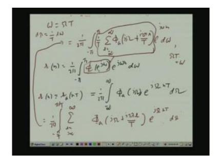
Capital omega its unit is radiant per second. Unit of time T is second. So, omega into T is just an angle radiant. So; that means, if I make the substitute in the integral then first you see when Omega becomes phi by T omega becomes phi. And when Omega becomes minus phi by T omega becomes minus phi. So, limits now of the limits of the integral now are from minus phi to phi.
