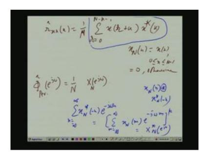
There you can now see this summation is a convolution between x and n with xn star minus n. So, discreet time fourier transform will be what convolution in time domain is prod prod multiplication in frequency domain. So, that means, phi cap period e to the power j omega which is the dtf t of discreet time Fourier transform r cap x as k. That will be what 1 by N,
