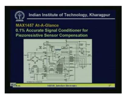
So now this is some chip in that direction temperature compensation chips are also available. Readymade chips which is maxim 1457 and which gives you 0.1 percent accurate signal conditional circuit chip for piezoresistor resistive sensor compensation.
