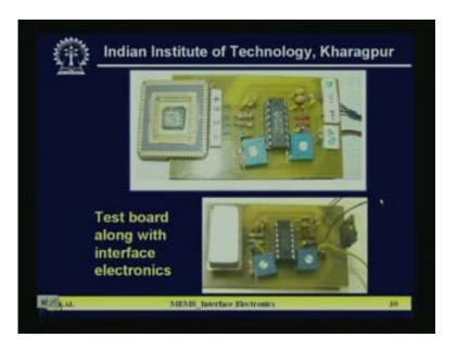
And that technique we have used in our case. In our accelerometer and here the circuits this, a TC 7652 is basically your chopper stabilized amplifier which has got advantage. Also in case of the offset cancellation 1 by f noise cancellation and along with that we have used 4 resistances to further reduce the offset value and that in a PCB package we have made along with accelerometer. Both this and this one are accelerometer on different packages and the circuit is the same.
