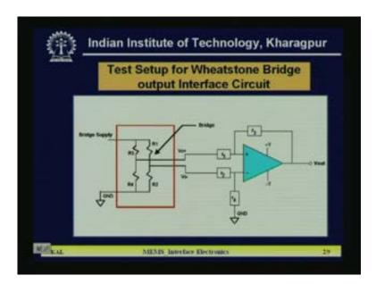
Now these are some of the simple circuits which can give you some offset cancellation also. That is the bridge output is connected with 4 resistances;  $R_1$ ,  $R_2$ ,  $R_3$ ,  $R_4$  and by adjusting these 4 resistances the offset voltage can be drastically reduced.
