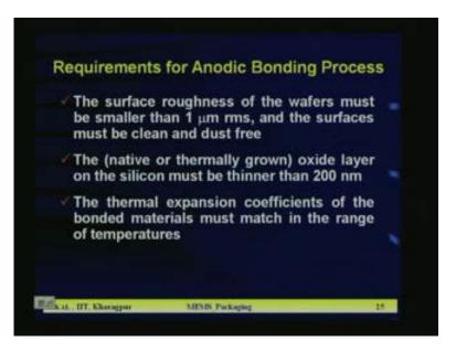
So others are surface roughness of the wafers must be smaller than 1 micron rms. So there in case of fusion bonding it was 10 angstrom. If you remember rms, but here roughly 1 micron rms is also the surface must be clean and dust free. The native oxide layer on the silicon must be thinner than 200 nanometer. Means 2000 angstrom the thermal expansion coefficients of the bonded materials must match in the range of temperatures.
