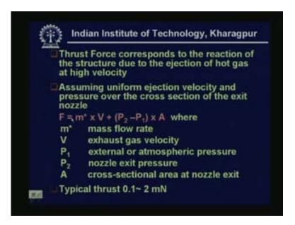
Now thrust force corresponds to the reaction of the structure due to the ejection for hit gas at high velocity. That we have to calculate and that is given by F equal to M star multiplied by V plus  $P_2$  minus  $P_1$  into A. Where M star is mass flow rate, V is exhaust gas velocity and  $P_1$  external or atmospheric pressure,  $P_2$  is nozzle exit pressure and A is construction area at nozzle exit. Typical thrust obtained out of this is 0.1 to 2 mill newton from this micro thruster.
