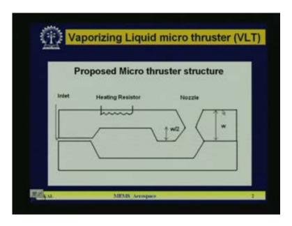
Now we propose a micro thruster structure which is very simple and homogeneous also. And there you can see is an inlet is here. This is the heating resistance and is nozzle and the top loop what will be the size optimum size that you have to have to choose. We have to select and what will be chamber size that is also selected. So a structure like this can be made very easily in the laboratory. So here top wafer we use diffuse, we just fabricate diffused resistors of 50 ohm.
