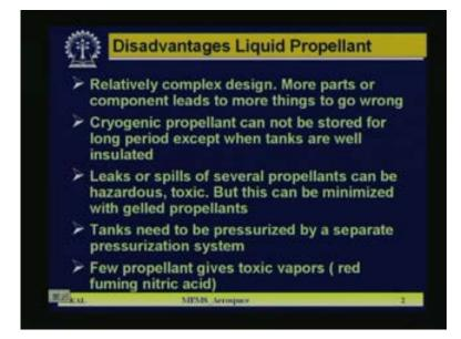
Now disadvantage of liquid propellants are these. A relatively complex design more parts are component leads to more things to go wrong. Since it is a complex a lot of parts will be assemble and any of the small parts may wrong which will compel us to leave the complete module.
