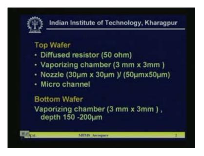
Vaporizing chamber is 3 millimeter by 3 millimeter nozzle is 30 micron by 30 micron. Micro channels will be there, bottom wafer is vaporizing chamber 3 millimeter by 3 millimeters depth will be 150 to 200 micrometer.
