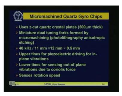
So here we use z-cut quartz crystal plates of 500 micrometer thick. The miniature dual tuning fork formed by micromachining. Photolithography anisotropic etching of quartz and the resonance frequency of the structure which we have designed is 40 kilo hertz. Natural resonance frequency of that every tuning fork is having some resonance
