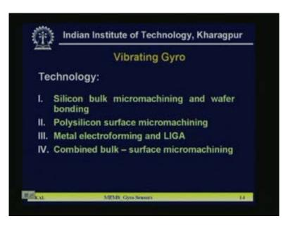
Now what are the technologies is used for vibrating gyro? They are silicon bulk micromachining and wafer bonding technology. Polysilicon surface micromachining which is a comb like gyros, metal electroforming and LIGA process is also used.
