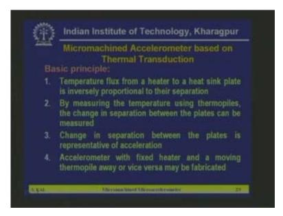
So these are the thermal transduction mechanism that also I told you a temperature flux from heater to heat sink plate is inversely proportional to their separation by measuring the temperature using thermopiles. The change in separation between the plates can be measured change in separation between the plates is representative of the acceleration. Accelerometer with fixed heater and a moving thermopile array or vice versa may be fabricated. That is not very much popular.
