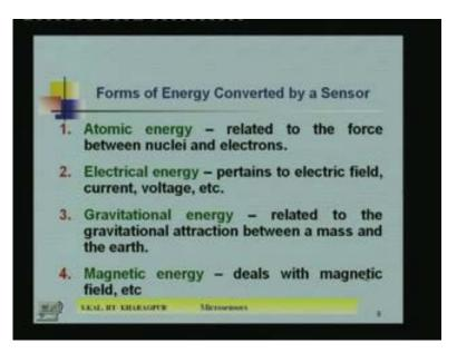
Now, what are the difference forms of energy converted by sensor? Those forms of energy are many. One is atomic energy, electrical energy, gravitational energy, magnetic energy and so on. So atomic energy relates the force between nuclei and electrons. So, that is the atomic energy. Electrical energy pertains to electrical field current or voltage. Gravitational energy it is related to the gravitational attraction between a mass and the earth. Similarly magnetic energy deals with magnetic field.
