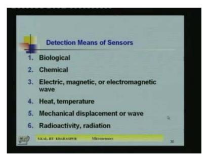
Now what are the detection means of sensors? Detections means may be biological, may be chemical, electric, magnetic or electromagnetic. Detection means may be heat or temperature, mechanical displacement or wave, radioactivity, radiation. These are various kinds of detection means.
