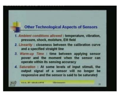
Now the other technological aspects of sensors, those are ambient conditions allowed. That means, what are ambient conditions: temperature, vibration, pressure, shock, moisture,
