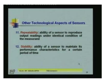
Now repeatability and stability are other parameters which you have to take into account when you are selecting or design a particular sensor. Repeatability means ability of a sensor to
