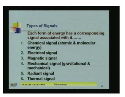
Now, what are the different types of signals we deal? Each form of energy has a corresponding signal associated with it. And those are chemical signal that is basically atomic and molecular energy, electrical signal, magnetic signal, mechanical signal which are gravitational and mechanical, radiant signal, thermal signal. So these are different signals we are getting and those signals are fed into your sensor system.
