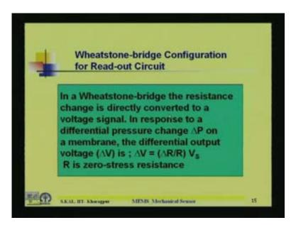
Now in Wheatstone's bridge, the resistance change is directly converted to a voltage signal. In response to a differential pressure, change delta P on a membrane, the differential output voltage delta V is delta V equal to delta R by R into  $V_S$  where R is a zero stress resistance. This is output voltage after the change of resistance because of the stress.
