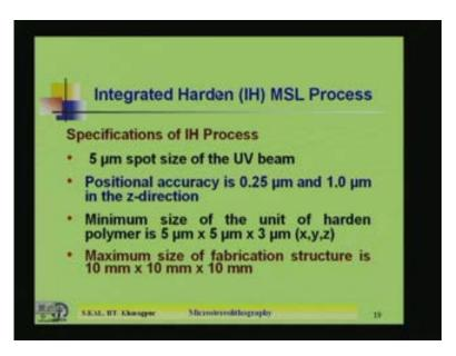
Now here what are the specifications of the IH process? 5 micron spot size of the UV system, positional accuracy is achieved to 0.25 micron and 1 micron in the z direction. Minimum size of the unit of harden polymer is 5 micron by 5 micron by 3 micron in xyz direction is the minimum size is possible. Maximum size of fabrication structure is 10 millimeter by 10 millimeter by 10 millimeter. So that is the maximum size of the complete structure.
