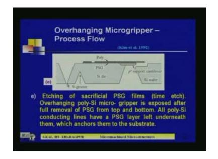
So in this way you can get the structure and you can separate it. So like this here if the etching of sacrificial PSG film time etches overhanging poly silicon microgripper is exposed after full removal of PSG from top and bottom. All poly silicon conducting lines have a PSG layer left underneath them which anchor them to the substrate.
