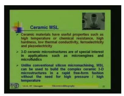
Now the ceramic MSL ceramic microstereolithography. These are some ceramic structure you can see at the corner of the figure. So ceramic materials have useful properties such as high temperature or chemical resistance, high hardness, low thermal conductivity, ferroelectricity and piezoelectricity. Because of those properties ceramic materials are used in some MEMS devices. 3D ceramic microstructures are of special interest in application such as micro engines and
