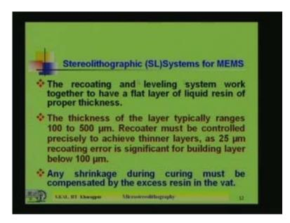
Now the recoating and leveling system work together to have a flat layer of liquid resin of proper thickness. Recoating and leveling because layer by layer you have to recoat after just recoating then leveling has to be done. That is done again by sensor electronic sensor.
