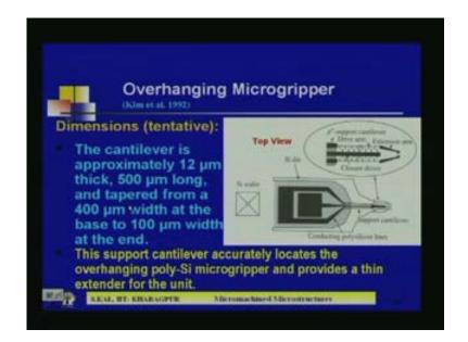
Now the tentative dimensions are shown here. The cantilever is approximately 12 micrometer, thick 500 micron long. This cantilever is a 500 micron long,12 micron thick and tapered from a 400 micrometer width at the base to 100 micron width at the end, so this is tapered. Here is a 400 micrometer and to coming here is a 100 micrometer. Here is a 400 and coming to 100. So if you go like this.
