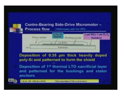
Heavily doped polysilicon pattern is to form the shield. That is completed deposition of first thermal LTO sacrificial layer and pattern for the busing and stator anchors. So that these anchors are here stator anchor and here you can see here.
