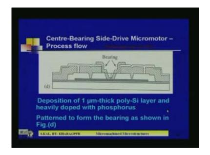
Here and then the bearing material is deposited 1 micron thick polysilicon layer and heavily doped with phosphorus. That patterned to form the bearing as shown in figure d. This bearing is found at the end step and then you will get the complete structure here.
