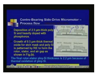
So deposition of 2.5 micron thick poly silicon is heavily doped with phosphorous. Poly silicon are heavily doped with phosphorous,growth of 0.5 micron thick thermal oxide for etch mask and poly silicon is patterned by RIE to form the rotor, stator and air gap as shown in figure b. So here you can see, so this is the thermal oxide here and now the mask polysilicon. There is patterned by reactive ion etching to get the separate becausehere the total thing is there. So this is LTO
