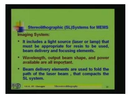
That is output beam shape and power available. That means it depends on the intensity. How much intensity is incident on the polymer, so those things are all important when you make the complete systems. Beam delivery elements are used to fold the path of the laser beam that compact the SL system.
