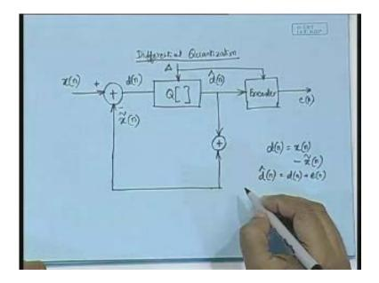
So d cap of n we can write as d of n plus e of n. What is e of n? e of n is nothing but the quantization noise. Then we can write x cap of n; x cap of n is nothing but x tilde of n plus d cap of n. This you have already said; so x tilde n plus d cap of n so both these will have a plus sign and here at this output we are going to get what we call as the x cap of n. So this is the x cap of n or in other words the quantized form of this x(n).
