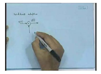
So if we are adopting the gain adaptation then the block would look like this that x of n and this we have to multiply by the gain which we are calling as G of n and this will be quantized. So it goes to the quantizer block Q and the output of the quantizer will be y cap of n and then it will be followed by the encoder and then we will be having the output codeword which is c of n and the output of this...... and this Q as well as the encoder will be controlled by the step size.
