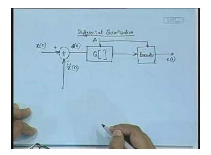
Now this is d of n and at the output of the quantizer we will call this as d cap of n. So this is the quantized version of the differential signal d of n. So this is d cap of n and now what we are doing is that d cap of n we are putting through a summer block. Now you see that if I add d cap of n with x tilde n what would you expect to get? x cap of n; because you see, now we can write down here very clearly that d of n is going to be x(n) minus x tilde of n. So definitely d of n if I
