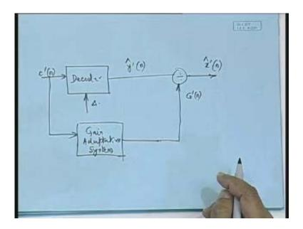
So this will be the decoder block diagram. You can see that the basic philosophy remains the same, only thing is that here we can derive it from c prime of n, very clear, we did not have to send the gain information into the channel.
