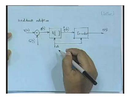
Now because it is a gain adaptation the step size delta will be constant and we have to take this output from the c(n). So based on the output codeword the gain adaptation system block will operate. This is the gain adaptation system (Refer Slide Time: 5:25) and the output of this gain adaptation would go to this multiplier block. So x(n) multiplied by G(n) will give us the y of n. this is the feedback adaptation.
