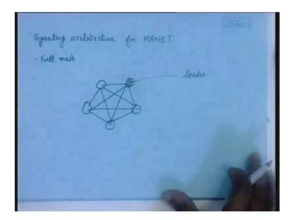
Now the difficulty about this is that such a kind of architecture is not scalable. Because if more number of nodes have to join in into this mesh obviously the signaling complexity will be very high because with more nodes joining in then it is not a scalable architecture anymore and in order to ensure scalability what we have is a kind of clustering architecture.
