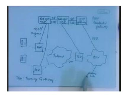
The thing is that in this case the use of SIP is actually restricted only within the IP domain whereas as far as the interfacing with the PSTN is concerned there a different signaling protocol is used but this way through this gateway configuration one can have a connectivity between the PSTN and the IP domain even if they use the SIP even though the SIP on its own is not supporting the interworking with the PSTN domain.
