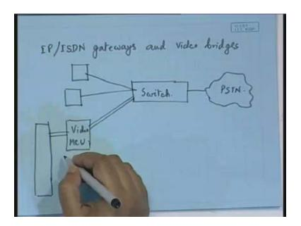
Now, because the MCU is the ultimate controller you need the MCU connected to this; not only eventually it should be connected to these terminal endpoints but also to the LAN. This is where I have LAN and then we should have an IP to ISDN gateway IP/ISDN gateway and the IP to ISDN gateway would again be connected to the switch so that one can establish ultimately a connectivity between the PSTN and the LAN.
