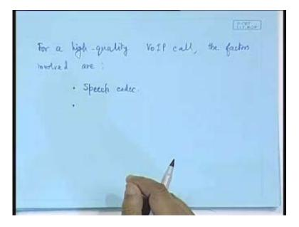
Then in this case, I mean, whenever we are transmitting the voice over internet the digitized samples what we have that has to be sent in the form of packets. Just like the way the data goes from one terminal to another; from the source to the destination the voice packets also travel in exactly the same way. So the scheme that utilize for the packetization that also dictates the quality of the VoIP.
