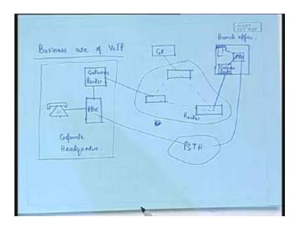
So here this is one configuration where you are making use of the IP as well as the PSTN based upon the congestion and based on the requirements you can choose either of the two routes. The other alternative way is that instead of connecting the telephones to the PBX why do not you connect the telephones to the LAN itself, those telephones are referred to as IP telephones.
