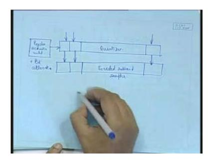
This is the flow diagram. I could not draw in one page this was the first page so we start with the filter bank then the frame buffer then the scaling is applied and after scaling, the samples are quantized, the quantization is decided by the psychoacoustic model and bit allocation and then we have the encoded subband samples. So this the flow diagram for encoding a frame of audio data.
