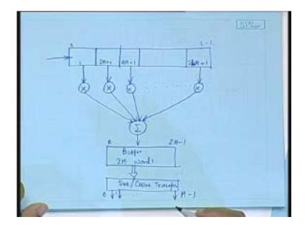
So these samples are the frequency domain samples what we are obtaining by windowing and sin cosine transform; so the same thing. What we had written down in form of the equation this is just an implementation of this and because this implementation basically involves modulating the center frequency of the filter by a factor of by an amount of pi by 2M or the odd multiples of pi by 2M that is how it realizes a polyphase filter.
