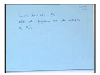
In that case this center frequency what we are talking of (Refer Slide Time: 20:25) this is going to be pi by M then this is going to be 3pi by M and this is pi and the bandwidth is going to be pi by M, so here to here we have pi by M or if you are taking from here to here that is pi by M.
