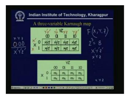
See that x y z the function is see the function is of three variable and we write in this way that is the function F of three variable x y z. Now, as it is a three variable, so what will be number of minterms what will be the number of minterms, the minterms will be 2 to the power 3 equal to 8 minterms. So, already we have discussed this will be x dash y dash z dash then x x dash y dash z like all eight terms will be there x y z.
