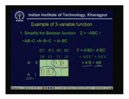
For a three variable function then simplify the Boolean function this A bar B C A bar B C bar A B bar C bar A B bar C. Now, I have to draw the Karnaugh map like that this is A bar A B bar C bar B bar C B C B C bar. So, the minterms exist A bar B C, so A bar B C means A bar B C this is one minterm, A bar B C bar A bar B C bar this is another minterm and the rest minterms are these.
