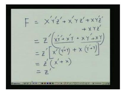
So, I have 1 function if that consists of x dash y dash z dash plus, the last term means x dash y z dash plus the x y dash z dash plus x y z dash see again that thing. So, this is x dash, y dash, z dash, x dash, y z dash similarly this is x y dash, z dash, because the for the second row x is the common literal and the last term will be x y z dash, now how we can reduce that thing, so how we can reduce.
