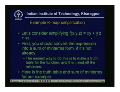
So, this is again a three variable function and the function is x y plus y dash z plus x z, so first we should convert the expression into a sum of minterms forms if it is not all ready. The easiest way to do this is to make a truth table for the function and then read off the minterms, so see how we can convert that thing, so first we will form the read table truth table see this is the truth table for the function given.
