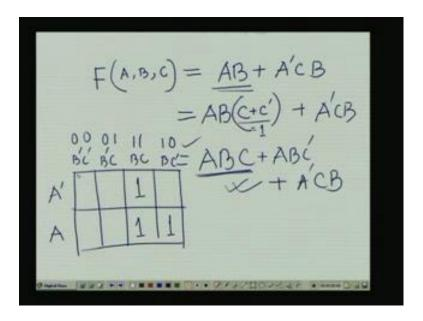
See what say one function F this is a A B C the three variable function, now it consists say A B plus A bar C B, so this two terms, now this what does it means A B, because it is a three variable function it means that one literal C that does not exist in the A B. So, I can easily introduce A B in such a way that C plus C bar, because A B means A B dot 1 and 1, I can always replace by C plus C bar and the remaining thing is there A dash C B.
