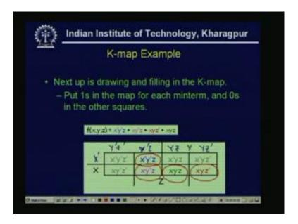
Again we are taking that three variable example, so put ones in the map for each minterm and zeros in the other squares that means, if I take a 1 function say here the function is x dash y dash z plus x y z x y dash z x y z dash plus x y z, so I will put 1, where this minterms exist. So, see that this is a x dash, so x dash and this is my y dash z dash this is my y dash z y dash z this is my y z and this is this is my y z dash.
