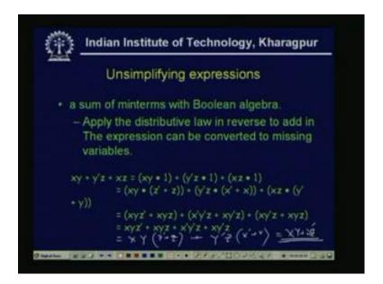
We can do the further simplification here that we can take x y from here we can take the x y common say x y then z dash plus z, here we can take y dash z is common then it can be x dash plus x. So, what will happen this becomes x y plus y dash z, so it is reduced to x y plus y dash z.
