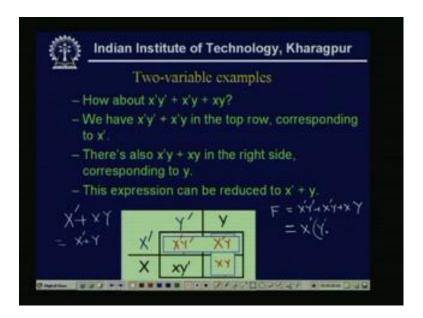
Now, my function consists of my function consists of, F equal to x dash y plus x dash y dash plus x dash y plus x y, now what are the terms from the in the map where it will be. So, we have x dash y dash plus x dash y in the top row corresponding to x dash, so called this is corresponding to x dash, so if I write this is my x dash y dash this is my x dash y and another term remains that is x y, so the another term is the second element of the second row and that is x y.
