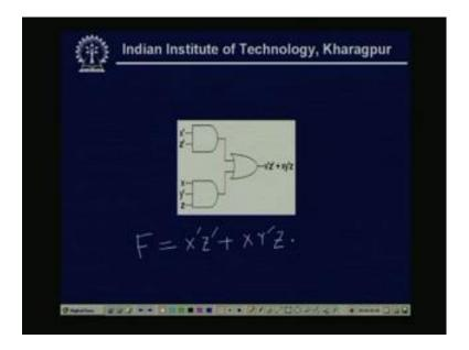
Now, see that here there is one circuit, simple circuit the two AND gate and one OR gate, and the input of the first AND gate is the x, so what this function realizes. The output Z realizes x dash x dash z dash means the complemented of x and z plus x this is a three input AND gate.
