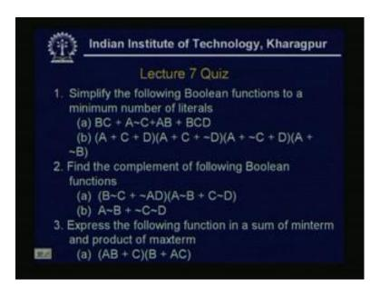
That simplify the following Boolean functions to a minimum number of literals, that means this is nothing, but the minimization of the Boolean expressions using the postulates and the theorems this is B C plus A bar A C bar plus A B plus B C D. And another expression is A plus C plus D, A plus C plus D bar, A plus C bar plus D, A plus B bar. So, just note that this is the sum of minterms and the next one, I have given is the product of maxterms and we have to simplify this thing.
