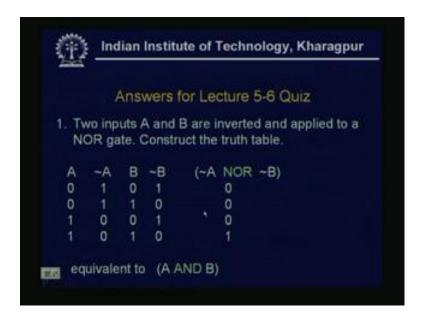
Now, A and B are inverted, so if A takes the values 0 0 1 1 this is complement of A 1 negation of A will be 1 1 0 0 it is inverted. Similarly, if B has the value 0 1 0 1 then negation B will be 1 0 1 0. Now, what will be the negation A and non-negation B, because these are the two inputs. See that, if negation A means 1 and negation B is 1 if we take OR 1 plus 1 then it will be 1 then complement of that will be 0. So, 1 plus is 1 1 complement of that becomes 0.
