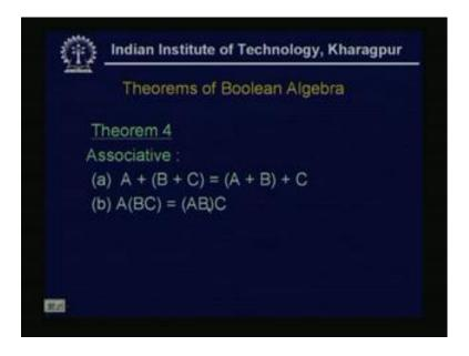
Now theorem 4, these are associative all ready we have seen that property the commutative when we have taken the two Boolean variables that A plus B is B plus A. Now, if it is three variable we take that means, A plus B plus C is if we take the operator operating on the first two variable A plus B and then on C plus C it will be same. Similarly, if plus is replaced by dot then A dot B dot C equal to A dot B dot C, so the
