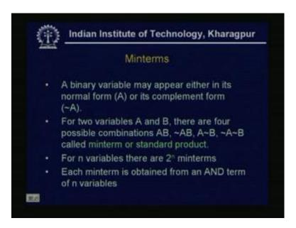
Now, we see the canonical and the and standard forms, before we define the canonical and standard forms first we define the mean terms, means terms and maxterms. So, a binary variable may appear either in its normal form just now, I mentioned A or its complement form negation A. For two variables A and B there are four possible combinations A B negation A B, A negation B negation A negation B.
