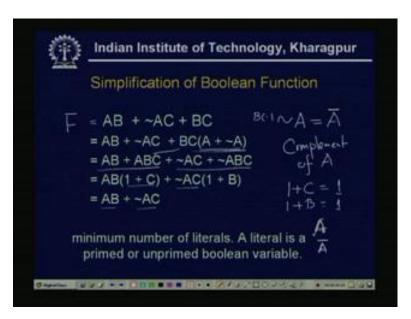
See I want to minimize or I am telling the simplification of some Boolean function, say I have 1 Boolean function A B plus A bar C mainly the negation AC. So, on negation A and this is same as, A bar these are all complement of A, so if I have 1 function say F equal to A B A bar C BC how we can simplify this thing. Now, I have I know the 4 postulates and the 6 theorems, now I have to apply this to simplify or to minimize this expression.
