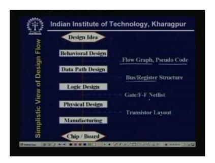
Now, although we give a very simple view of design flow, see this is a this is design idea means, the given the system to the implemented that the designer must have the idea that or a some abstract level design idea that how it can be implemented in hardware. So, that we are calling the design idea then, this whole design its behavior, the behavioral design is represented, this can be a how this can be represented. So this can be a flow graph or this can be a pseudo code.
