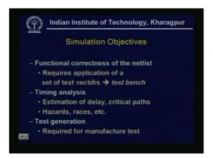
So, simulation objectives are functional correctness of the netlist, this requires application of a test vectors, we apply or test vector to some test bench, we have to generate. Then, timing analysis the estimation of delay critical paths, whether Hazards are there, above added races conditions are in overcome and the test generation this is required for manufacture test. So, these are the simulation objectives.
