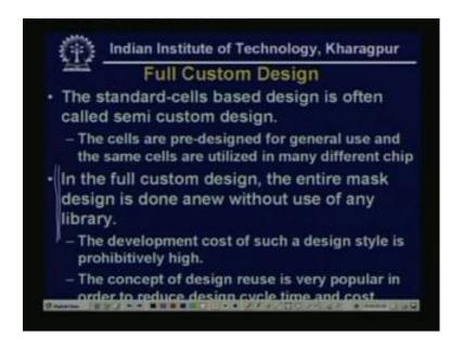
Now, is the full custom design, so the standard cell based design is often called the semi custom design. The cells are pre-designed for general use and the same cells are utilized in many different chip. In the full custom design the entire mask design is done a new, without use of any library, so this is very important that actually from such, we have to design, there is no cell library available.
