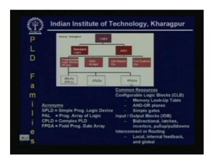
Now, these are programmable logic devices, already we have read the, how these PLDs means the PAL. PLA they can be designed, they can be, what is the actual circuitry of the PAL or the PLA. Now, using this programmable logic devices, this can be the systems or this VLSI circuits can be implemented. Now, the logics are normally of two types, standard logic and ASIC.
