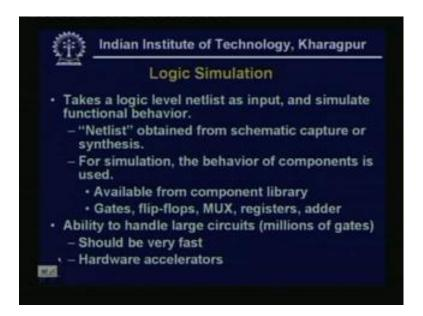
Now, the third step is logic simulation, so this takes a logic level netlist as a input and simulate functional behavior and netlist obtained from schematic capture is the actual circuitry or synthesis, for simulation the behavior of components is used. Now, these are available from component library, gates flip flops MUX registers adders these are my equipments which are necessary for my logic synthesis and we knew, we know the how or the truth table of these gates.
