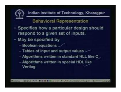
Now, see how this behavioral representation can be done, so behavioral is representation it specifies how a particular design should respond with given set of inputs, its behavior of a system. So, this may be specified by Boolean equations, already we have seen that given Boolean equations, how Karnaugh map can be kernel map synthesize the actual and or design and different type of other techniques we have seen that from Boolean equations to realize the actual hardware circuit.
