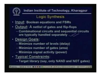
So, logic synthesis the input can be Boolean equations and FSMs, output a netlist of gates and flip flops, now combinational circuits and sequential circuits are typically handled separately. And in this class already we have seen that from the Boolean equations how they can, the circuit can be synthesized or the combinational circuits or different sequential circuits, how they can be synthesized, that part already we have read.
