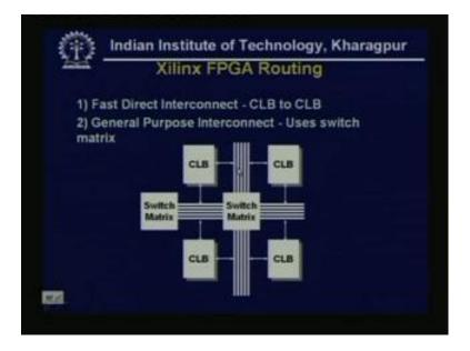
This is one Xilinx FPGA routing, so this is mainly the, the CLBs are there, the Complex Logic Block and mainly some switch boxes are there which are connected this logic box. So, this is the overall idea of the FPGA how this can be programmable, mainly they are
