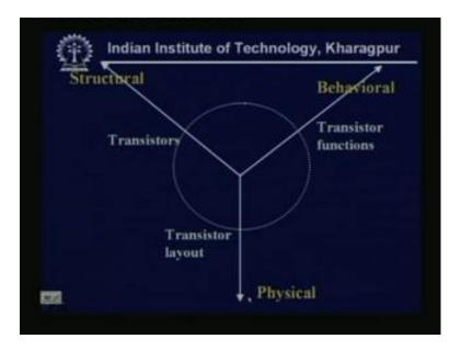
Now, the structural thing can be realized by transistors, again the behavioral things can be the transistor functions and this can be transistor layout. So, ultimately we want the implementation of transistors on silicon and that is my physical thing.
