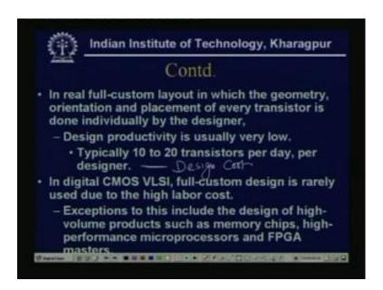
So, in real or like full custom layout in which the geometry orientation and placement of every transistor is done individually by the designer. So, design productivity is usually very low, typically 10 to 20 transistors per day per designer, so cost is high. Here the cost, design cost is very high, design cost is high.
