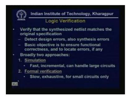
Then, another is logic verification, so it verify the synthesized netlist matches the original specification, detect the design errors also synthesis errors, basic objective is to
