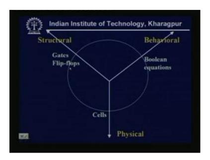
So, structures even the structures can be gates or flip flops ultimately, it should be gate and then that gate can be realized by transistors. And behavioral can be Boolean by
