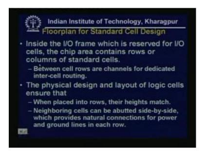
Now, floorplan for standard cell design, so inside the I O frame which is reserved for I O cells the chip area contains rows or columns of standard cells. Now, between cell rows are channels for dedicated inter cell routing and the physical design and layout of logic cells ensure, that when placed into rows their heights match, neighboring cells can be abutted side-by-side which provides natural connections for power and ground lines in each row.
