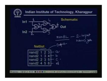
We take one example, say we take one simple circuit, this is a 4 NAND gate, I give some line number, so this is a input 1 and that line is represented as a 1. Similarly, input 2, input 2 is 2, this intermediate line is 3, some numbering I am giving this is 4 this is 5 and the output line is 6. So, the netlist will be the, how they are interconnected that information should be there, so all are 2 input NAND gate and that can be represented as a NAND 2.
