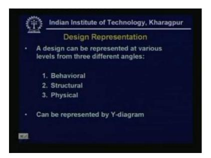
Now, first thing we see the design idea, how that can be represented we call the design representation, so design can be represented at various levels from three different angles. It can be behavioral, it can be structural, it can be physical, now this three can be represented by the very popular Y diagram.
