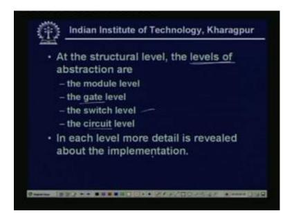
Now, at the structural level the levels of abstraction are module level, gate level, switch level or circuit level. If it the very large circuit; obviously we cannot represent this thing by a NAND gate or AND gate, so this can be module level. Now, this module is a set of that can be a set of gates or even set of sub modules and this sub modules are actually realized by set of gates. So, that is why the, they are the, there are different levels of abstraction.
