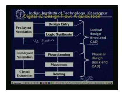
Now, we see the, the actual digital IC design flow; that means, when the circuit becomes very large then how they can be automated using the CAD tools. What are the different steps to be followed? So, first is the design entry or just now the thing we have
