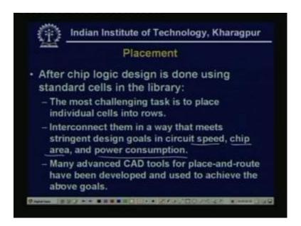
Now, the placement actually now, actually the, the physical design portion, that after chip, logic design is done using standard cells in the library, the most challenging task is to place individual cells into rows where the rows should be placed. For that the interconnection length will be minimum; that means, the routing cost should be minimum and parallely the delay the, the area, area should be minimum.
