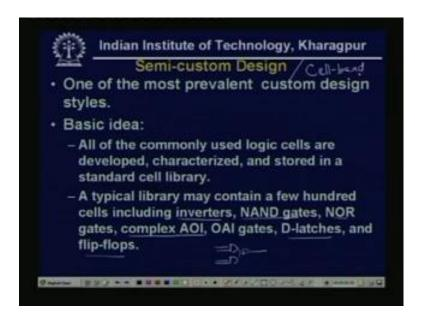
Now, the secondary one is semi-custom design that one of the most prevalent custom design style, the basic idea is all of the commonly used logic cells are developed, characterized and stored in a standard cell library. Nowadays for digital design, the moderately complex or very complex digital systems, this is the state of the art, that the logic cells they are developed, characterized and stored in a standard cell library.
