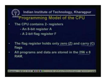
So, now first we assume the programming model of the CPU, the CPU that we want to design contains two registers, an 8-bit registers A, a 2 bit flag resistor F, the flag register holds only 0 and carry C flags. All programs and data are stored in a memory and the memory size is a 256 by 8 bit RAM, now the first we see the hardware schematic of the data flow part of this processor.
