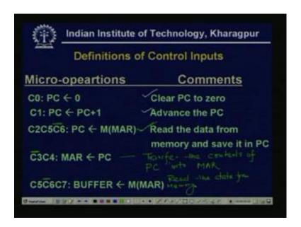
Now, we define the control inputs first C 0 to C 9 the these are the micro operations, what are the micro operations for these control signals and what are the meaning of those micro operations. So, first one is C 0, the C 0 is micro operation is 0 assign to PC or PC is reset or PC is clear, so clear PC to 0, so C 0 is clear PC to 0. The control signals C 1 activates the operation, which is defined as PC is PC plus 1 means the program counter value is incremented by 1.
