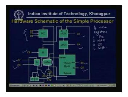
So, it is the Program Counter or PC, MAR the Memory Address Register, IR the Instruction Register and buffer, so these four more registers are also there. So, in addition with A and F, the four more registers are PC Program Counter, Memory Address Registers MAR, Instruction Register IR and a buffer. These registers are transferring to a programmer that, 8 bits registers buffer is used to hold the data that is, retrieved from the memory.
