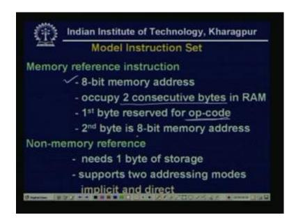
As I defined, that they need a memory address in this example, we have assumed that then they need an 8 bit they occupy 8 bit memory address. They occupy, the memory reference instruction occupy two consecutive bytes in RAM, the first byte reserved for op code and the second byte is 8 bit memory address. So, op code and address, these two are, are the two content of the two bytes occupied by memory reference instruction.
