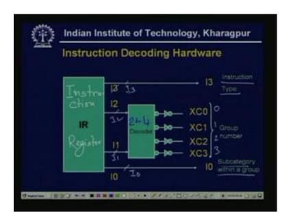
Normally, the first step is only called the fetch cycle, the fetch instruction is normally called the fetch cycle and remaining instructions, this is called the fetch cycle and remaining from step 2 to step 6, these are called execution cycle, is a execution cycle. Now, how to decode the instruction, so we see the hardware for instruction decoding, see this is the Instruction Register IR, this is my Instruction Register.
