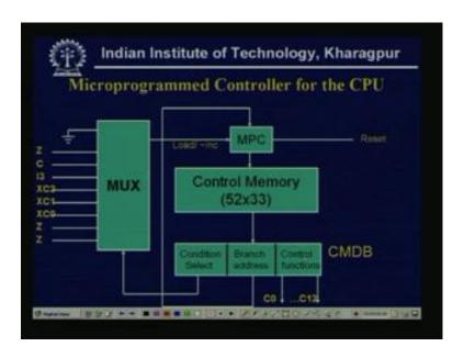
For this example CPU, will be seen that there is a multiplexer, this is a the MPC, the control memory and the CMDV that actually these are the register where three fields are they are condition select branch address and control functions that already we have seen. So, now what we have to do, that the symbolic micro program, that implements the instruction sets.
