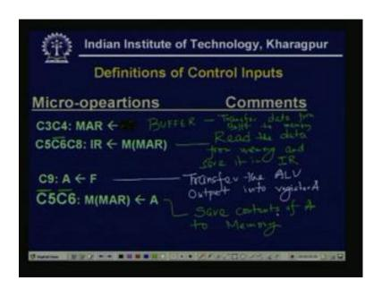
Then, C 3 C 4 if we see C 3 C 4, C 3 C 4 is buffer or C 3 C 3 complement C 4, first we see C 3 complement C 4 then, the PC goes to MAR. Then, transfer the contents of the PC into MAR, if it is C 3 C 4 if we see, if it is C 3 C 4 then, it will be buffer to MAR, this
