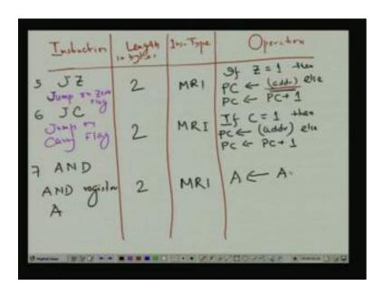
Now, in this way that we can write the other instructions, quickly we can write the other instructions, again length in bytes, instruction type then operation. So, jump on 0 and jump on carry, there are of jump type, jump on zero flag set, this is a, this is a jump on zero flag and this is a jump on carry flag set. That means, if there 1 if Z equal to 1, if C equal to 1, both are of MRI type.
