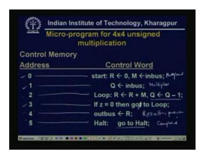
Now, the design of a programmed control unit, we consider, and the example we have taken, is the same example of that, hardware control unit, we have consider a 4 by 4, unsigned multiplication. So, this is 4 by 4 unsigned multiplication, the technique is repetitive addition, so here the, as it is a memory, so there will some address, and some content. So, the control memory address, say we give the control memory address are 0, 1, 2, 3, 4, 5 as there are six micro instructions.
