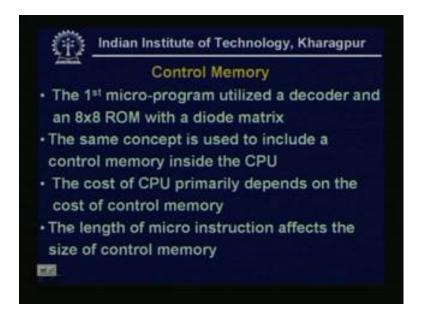
Now, this, the memory, which contains this program, micro-program, we call this is control memory. Now, we see, what will be the features, of this control memory or how actually the control memory is being accessed, or how it is written, written data on to it, now if the concept of micro-programming was first proposed by, W V Wilkes in 1951. So, when first it was introduced, the micro-program, utilized a decoder, and an 8 by 8 ROM with a diode matrix.
