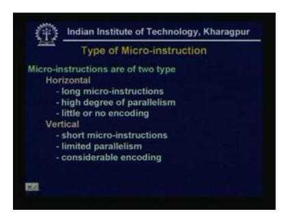
Now, we see that the different type of micro-instructions, so micro-instructions are of two types, one is called horizontal and another is vertical. Now, the horizontal micro-instruction mechanism provides, long micro-instruction, a high degree of parallelism and little or no encoding. Whereas, the vertical micro instruction it, offers short micro-instruction, it as limited parallelism, but it has considerable encoding.
