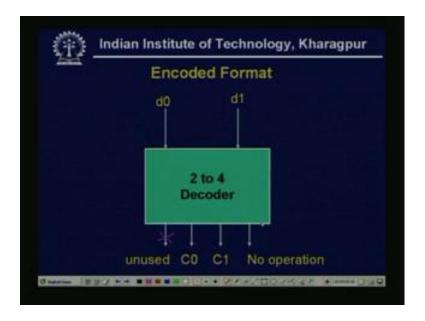
So, the implementation of encoded format is like that, only d 0, d 1 will be the input of decoder, and the outputs will be that, two will be the actual control signals, like in this example C 0, C 1, 1 is no operation. Actually, there are operations, if we include the no operation, itself is NO is one operation, and one line is unused, so this unused, so this, the implementation of encoded format, using decoder.
