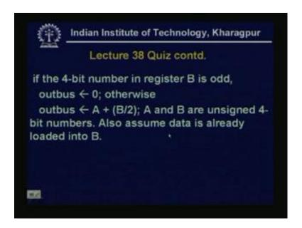
And, the operations are like this, if the 4 bit number in register B is odd, then 0 is assign to out bus, otherwise out bus is A plus B by 2, A and B are 4 bit numbers. And, we assume, data is already loaded into B, so this is the quiz of this particular lecture, and here, we finish this class.
