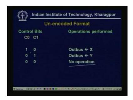
See, first we consider the un-encoded format, un-encoded format, so this is the normal see a simple situation, that when each control bit is 1, 1 operation is performed. So, C 0 is 1, C 0 is 1, X is assign to out bus of the content of this register, goes to the out bus, if C 1 is 1, content of Y register, goes to the out bus. If all are 0, C 0, C 1 is 0 their will be no operation. So, these three operations can be d1, by specifying the control bits C 0, C 1 as 1 0, 01, and 00.
