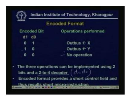
Now, the same thing can be d1, in different way, in a, encoded format, see as it is encoded format, so here, the relationship are like that, say this, these are some bits, this d 1, d 0. See, if we consider a, these 3 operation, we implement using 2 bits, and a 2 to 4 decoder, so as if d 1, d 0 of the inputs of this decoder. Now if d 1, d 0 is 0 1, X contents of X goes to out bus, if it is 1 0, contents of Y goes to out bus, if it is 0 0, then there is no operation
