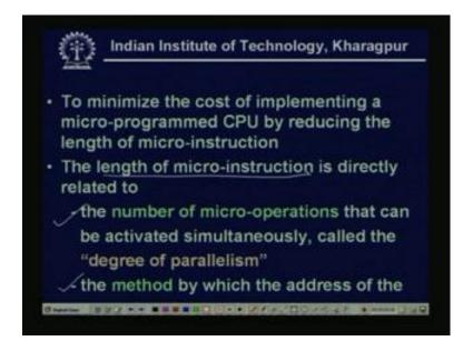
Now, to minimize the cost of implementing a micro-programmed CPU, reducing the length of micro-instruction is needed. Now, the length of micro-instruction, is directly related, to the number of micro-operations that can be activated simultaneously, call the degree of parallelism. As the program is a set of instruction or micro-operations, so in every program, there are some, a, some of the micro-operations can be performed, simultaneously.
