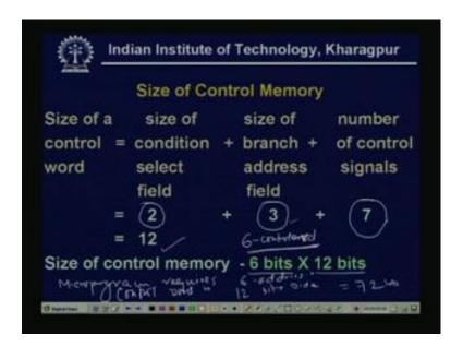
So, we see what will be the size of control memory, see size control word, should be size condition select field, size of branch address field, and number of control signals. So, just now we have seen, the number of control signals are, 7, and size of condition select field, size of condition select field is 2. Now, there are 6 control memory address see, just we have seen, there are 6 control memory address, 0 to 5 are required, for the control memory to store the micro-program.
