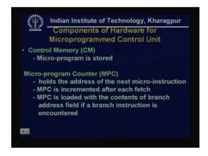
First is control memory, this is the main component of the design, and it stores, the micro-it contains the micro-program, so the micro-program is stored here. Now, next one is the micro-program counter, it is called MPC, it holds the address of the next micro-instruction to be executed. Now, MPC is initially loaded, from an external source to point to the starting address of the micro program, the MPC similar to program counter, so MPC is implemented after each fetch.
