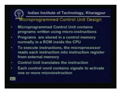
So, first we see, what we mean by, micro programmed control unit, and then we will read the, design of that type, particular type of control unit. Now, micro programmed control unit contains the programs, this program is nothing but, a set of micro-instructions. Now, programs are stored in a control memory, normally in a ROM inside the CPU, now to execute instructions, the microprocessor first fetch each instruction, in to a instruction registers, from external memory.
