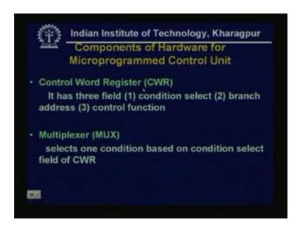
Now, the control word register or CWR, so control word register, each control word in the control memory, is assume to contain three fields, one is condition select, branch address and control function. Each micro-instruction, fetched from control memory is loaded in to CWR, the control word register, now the organization of the CWR is same. For each control word, and contain, the three fields, these three fields condition select branch address and control function.
