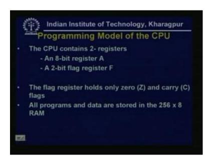
So, now first we assume, the programming module of the CPU, The CPU, that we want to design contains 2 registers. An 8 bit registers A, A 2 bit flag register F. The flag register holds only 0, and carry C, carry C flags, all programs and data are stored in a memory, and the memory size is a 256 by 8 bit RAM. Now, the first we see, the hardware schematic of the, data flow part of this processor.
