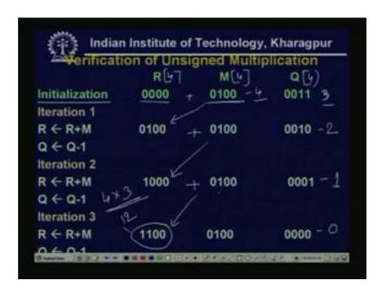
Now, how do we verify, second thing was validate the, the flow algorithm, a verification of unsigned multiplication. So, we have 3 registers R M Q say these are 4 bit registers, R M and Q, then initialization we take some actual data, say R is initially set to 0, so all 0, M is 0 1 0 0 means, decimal value 4. And Q is 0 0 1 1 means, the decimal value 3, now in iteration 1, R is R plus M, so it was, earlier these 2 will be added, and result is here, so all 0 plus 0 1 0 0, this is 0 1 0 0.
