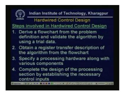
First we see, that what are the steps involved, in hardware control design, now the step 1 is, derive a flow chart, from the problem definition and validate the algorithm, by using a trial data. So, given a problem, the first we derive the flow chart and flowchart means,
