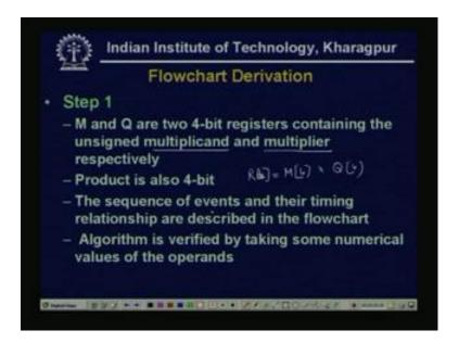
Now, the step 1, using this example the 4 by 4 multiplier, simple multiplication then we 1 by 1, we see that how the steps of the hardware control design is followed, and we can get a actual implementation of the control unit. Step 1 was, derive a flowchart from the problem definition and validate, the algorithm by using, that trial data, see M and Q are, 2 4 bit registers, obtaining M and Q are 2 4 bit registers, and they contain the multiplicand, and the multiplier respectively.
