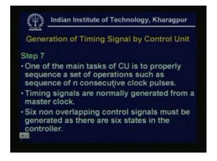
Now, step 7 the general of time signal by control unit, see one of the main tasks of CU is to properly sequence a set of operations, such as, sequences of n consecutive clock pulses. And timing signals are normally generated from a master clock, so six non overlapping control signals, must be generated, as there are six states in the controller.
