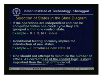
Now, one should not, attain to minimize the number of states, as correctness of the control logic is more important, than the cost of the circuit. So, for the first case for the initial design of control unit, we will not minimize the number of states, as it is a machine, so we can run, we can do the state minimization. But, as correctness of the control logic is more important, that is, that is here, our M is not the actually, the minimization, but to get the actual correct design of the CU.
