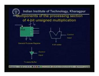
So, this, components are like that, one is the general purpose register, so this is the general purpose register. One clock is there, this is a 4 bit input, 4 bit output, and these are the three inputs C L and D.
