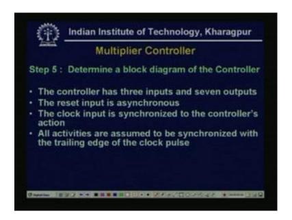
Now, step 5, determine a block diagram of the controller, now, the controller has three inputs and seven outputs, the reset input is asynchronous, the clock input is synchronized to the controller section. All activities are assumed to be synchronized, with the trailing edge of the clock pulse, so this is my step 5.
