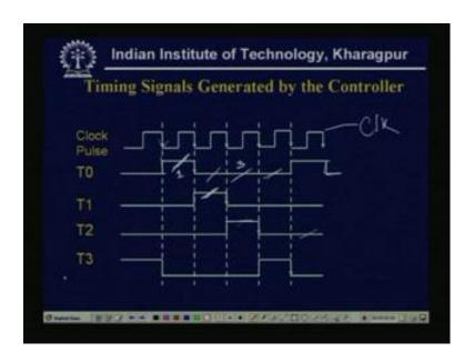
Now, we see one example that how the timing signals, are generated, see, we have, one we have 1 master clock pulse. So, there are six states in the controller state diagram, so six non overlapping timing signal T 0 through T 5, must be generated. So, that only one will be high, for a clock pulse. Now, here we have, shown that 4 timing signals T 0, T 1, T 2, T 3 say this is a master clock pulse, this is my master clock pulse.
