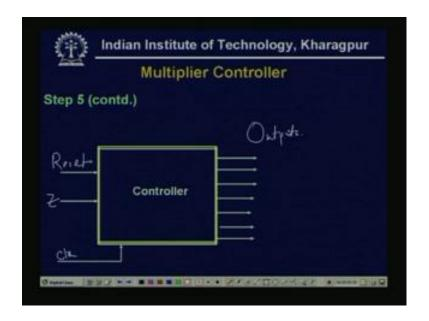
So, what will be the controller design, so controller has one input is reset, controller one input is reset, this is a Z input, this is a clock. And seven outputs, these are seven, these are the outputs.
