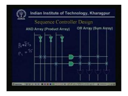
So, if it is a PLA design, then this type of AND array, and OR array circuits will be there. And the logic, we can write, that of the product term is generated in the PLA designs as P 0 plus Z bar T 3, and P 1 equal to T 5. P 0 equal to Z bar T 3 and this is P equal to T 5, and then, this the output signals will be generated. So, and we have seen, that in this way, we can design the control circuits.
