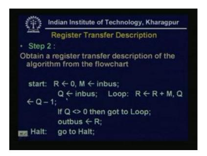
Now, step 2; step 2 was obtain to register transfer description of the algorithm, from the flowchart. So, again using the same example of multiplication, R is set to 0, M is in bus, Q is assign to the data of in bus, and then, this loop is R is R plus M, Q is Q minus 1, if Q not equal to 0, then go to loop out bus is R halt go to halt. So, actually what, algorithm we, we have decided, the algorithm we have read, it is there, in the register transfer logic.
