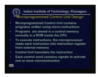
So, first we see, what do we mean by, micro programmed control unit, and then, we will read the design of, that type, particular type of control unit, Now, micro programmed control unit, contains the programs, this program is nothing but, a set of micro instructions. Now, programs are stored in a control memory, normally in a ROM inside the CPU, now, to execute instructions, the microprocessor, first fetch each instruction into instruction registers, from external memory.
