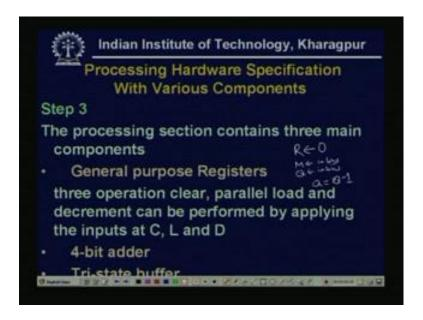
Now, the step 3, the processing section, step 3 was specify a processing hardware along with various components. So, the processing section contains, three main components,
