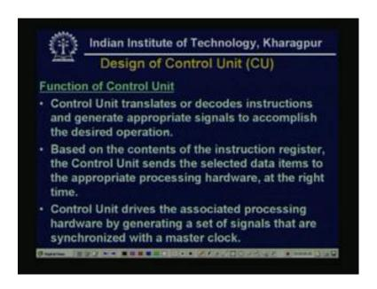
So, control unit translates or decodes instructions and generate appropriate signals to accomplish the desired operations. So, you have read the design of instruction set there the instruction is fetched and then it is decoded. So, after this decoding is done by the CU the control unit and then it generates appropriate signal for performing that particular operation defined by the instruction.
