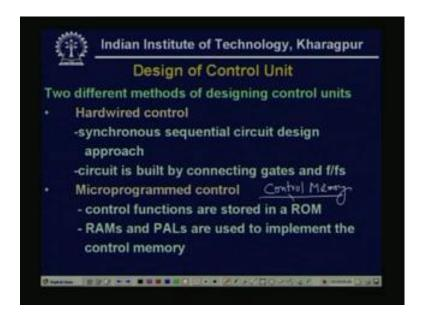
Now, we see that how this control unit, so how this control units are designed can be implemented. We have seen that these are the functions mainly the instruction interpretation phase, some functions it has to be performed and the see instruction sequencing part.
