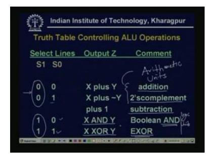
So, if we see the truth table controlling the operation if this ALU, so this is a truth table. So, I have two arithmetic or my arithmetic unit consists two functions, one is addition another is subtraction the 2's complemented subtraction.
