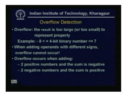
So, how we can detect the overflow, the result is too large or too small to represent properly. And example is just now we have seen when adding operands with different signs overflow cannot occur. Now, overflow occurs when the two positive numbers is a very important thing that two positive numbers and the sum is negative or other cases two negative numbers and the sum is positive. So, just now we have seen the two examples of each of the cases.
