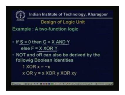
Now, we see two function logic, earlier we have seen two function arithmetic unit. Now, we see a two function logic logical unit, see in the example last example if S equal to 0, then it was a AND, if S equal to 1, then it was a sub tractor. Now, we are checking we are designing AND logic that if S equal to 0. That means, select line of the multiplexer is 0, then the function G is X and Y else the function is X XOR Y either it is doing AND or
