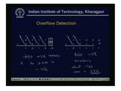
Each of the cases, how we can detect the overflow, these are the two cases that this is two positive numbers 7 and 3 two positive numbers and there is sum is negative. Here, two negative numbers and the sum is positive, so both the cases the overflow occurs.
