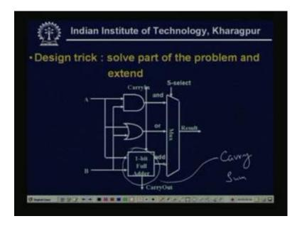
So, design trick is solver part of the problem and extended. That means first 1 bit full adder is designed, it has two parts the carry and sum. Just now we have seen we have design and then the other logics the one AND gate and one OR gate that we can do.
