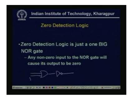
Now, zero detection logic, so zero detection is just a one BIG NOR gate. Any non-zero input to the NOR gate will cause its output to be 0, because NOR is complement of OR is that if anyone at least if 1 bit is one input is 1,then it will be output will be 1. So, NOR is that if 1bit is 1 is actually my NOR gate, so anyone is 1, then it will be a 0, so that logic we can use for a zero detection.
