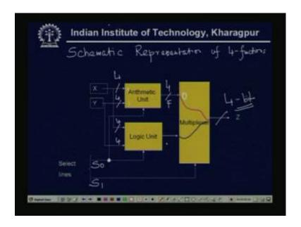
So, if we see the schematic representation, whatever be the unit, just as an example we have seen very small two function arithmetic units, addition and subtraction and two functional logic units the AND and the XOR.
