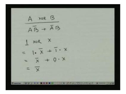
Say if it is A XOR B, we know the truth table of this thing is actually function is AB bar plus A bar B. So, 1 XOR X means 1 and X bar plus 1 bar dot X. Now this is nothing but X bar plus 1 bar is 0, so this portion will this is ended with 0 means nothing will be there. So, this is a X bar
