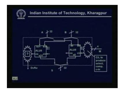
Now say, we have taken the two ALU and actually we are considering overflow, so if it is a 32 bit, A is the 32 bit, B is 32 bit and we are taking that 32 such ALUs that 1 bit ALU we have kept here. So, A 0 to A 31, so here some ALUs are there, A 0 to A 32, similarly B 0 to B 32 are fed. And these are the select lines, S 0 to S 31, and it produce that the combinational logics to produce select compare the carry in etcetera.
