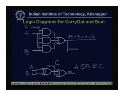
Now, say the one full bit for the full adder this is the logic diagrams for carry out and sum already we have several times we have read. We have the design of full adder and we know that this is the A if AB are the two inputs and is another is the carry in say a C, then we know that AB plus BC plus CA that is my AB plus BC plus CA is my carry out. So, this is the simple logic diagram
