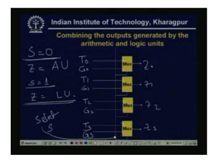
So, what we can do, say the T 0 T 1 T 2 T 3, the output of the arithmetic units come to that first line the zeroth line. Similarly, the G 0 G 1 G 2 G 3 comes to the multi other multiplexer inputs and as usually it has some select lines, it has the select lines S.
