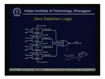
So, again if we use a 1 bit ALU just there are 4 bit ALU A 0 B 0 A 1 B 1 is given and the four outputs result are this is simply a NOR gate, So, you A 0 at the output gives a A zero detection.
