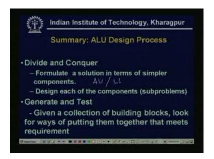
So, if we to the summary the of the ALU design process that there are two main concepts one is divide and conquer; that means formulate a solution in terms of simpler components. So, if it is a ALU means either arithmetic units or logic units that first we will be designed using gates or our simple gates.
