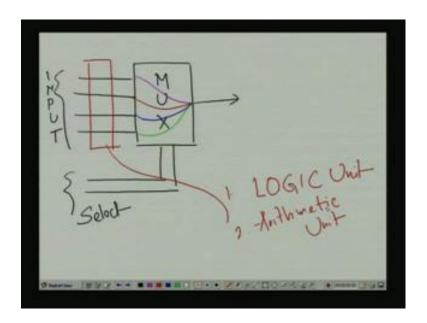
And, if we have a four function Logic units or four function arithmetic units we need, then actually the way. What we can do, we can take a multiplexers which have four input lines two select lines and the accordingly that particular output can be selected. These are my input lines and here these, what we can do that here, this can be this red box, this can be a LOGIC unit or this can be an arithmetic unit.
