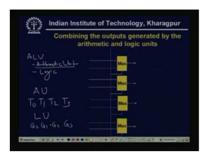
Now, we can combine the outputs generated by the arithmetic and logic unit as the ALU consist the, or ALU is has two parts, one is arithmetic unit and the logic unit. And just now, what we have done, the two way or two function arithmetic units and add and subtract we have designed two function logic unit AND and XOR we have designed.
