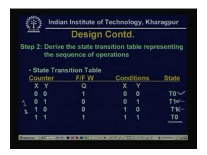
Now, the second step is the derive the state transition table representing the sequence in sequence of operations, so the state transition W, we see that the counter, then it is a W flip flop, the conditions and then, what will be the state. So, if it is 0 0, the flip flop value is 1, conditions to be checked is 0 0 and state is T 0.
