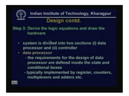
Now, the third step is deriving the logic equations and draw the hardware System is divided into two sections the data processor and controller. So, the data processor the requirements for the design of data processor are defined inside state and conditional boxes and typically these data processors and implemented by the digital components like registers, counters, multiplexers and adders etcetera.
