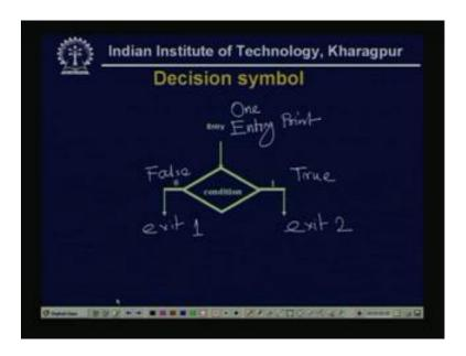
Now, symbol is here this is the one entry point and there are two exit, so if the condition is false, then this is one exit 1, if the condition is true, then it is a exit 2. So, there are two exit point, sometimes another decision symbol is used that is a hexagon.
