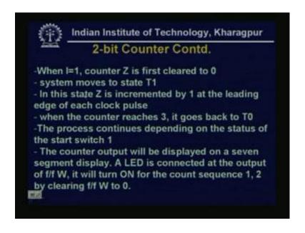
Now, some more specs that, when I equal to 1 counter Z is first, clear to 0, system moves to state T 1, in this state Z is incremented by one at the leading edge of each clock pulse, when the counter reaches 3, it goes back to T 0. So, it will be all the term, it will be 0 0, if it is only it counts 1 and 2, that will it will change 0 1 1 0, again you when it will be 1 1, it goes back, the process continues depending on the status of the start switch 1.
