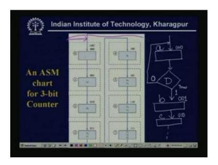
Now, we take one example of an ASM chart for a 3 bit counter for a 3 bit counter this is a mod 8, so it has 2 to the power three states, eight states, if the state symbols or the logical name is A, B, C, the three things. Then, actually that it will be 0 0 0, 1 0 0 1, 0 1, 0 like that it will goes to 1 1 1, now before that... That means, the input should be like will be first, it will go to a state symbol, say this is A B C and code is 0 0 0.
