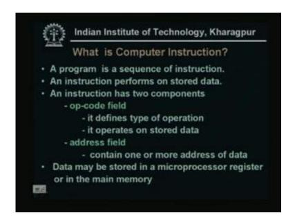
Now, before stating the design, what do you mean by computer instruction, all of you know that, a software program is consist of a sequence of instructions. Now, an instruction performs on stored data that means a program is nothing but a sequential operation to be performed on the data and an instruction is one single operation on the data.
