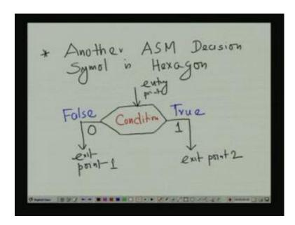
Normally, another type of ASM decision symbol is hexagon, normally 1, again, here one entry point and two exit point, this is the condition, if it is false a 0, if it is 1, means true. So, this is the entry point and there are two exit points, so normally these are the three symbols, ASM symbols are used to represent the ASM chart.
