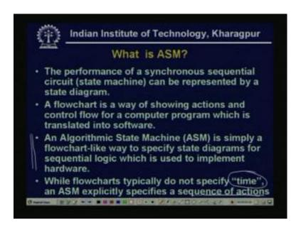
So, first we will see what is ASM, what do we mean by algorithmic state machine chart, before that we again we recapitulated the synchronous sequential design. The synchronous circuit, normally it is made up of the combinational circuit with the memory and the memory is a clocked flip flops. Now, the performance of synchronous sequential circuit or simply we can tell the state machine can be represented by a state diagram.
