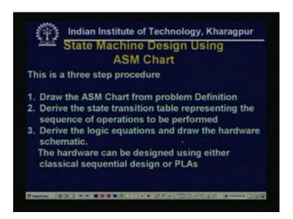
Now, we see that, what are the generic steps for the state machine design using the ASM chart, normally this is a three set procedure, the first step is the draw the ASM chart from problem definition. Problem definition means just now that machine specification I told, that one register X is there a flip flop A is checked, if it is 0, then go to a state T 1, if it is 1. Then, increment X by 1 and next state will be T 2, so this is my problem definition of the problem specification.
