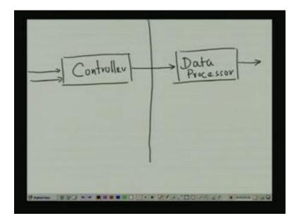
What, we have see that, if we draw that, it has two part, one is the controller, another is the data processing, the inputs are here and the after processing the output, so actually there will be a partition here. Now, for this particular example of 2 bit counter, that data processor part is the 2 bit counter, Say the 1 2 input AND gate, the flip flop, W, these three constitutes a data processor parts, so these three are the data processor.
