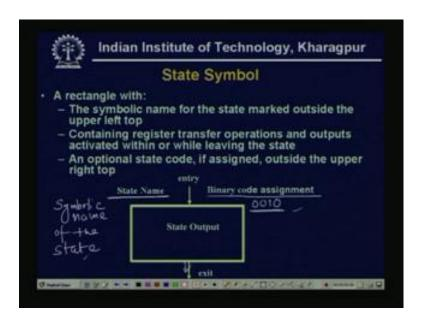
Now, first receive the state symbol, it is a rectangular shaped, now here one state name should be there and the binary code assignment, say if it is a 4 bit say 0 0 1 0, this type of binary code is assigned here. It has one entry and one exit, normally this is the state output, so it is a rectangle with the symbolic name for the state marked, outside the upper left top.
