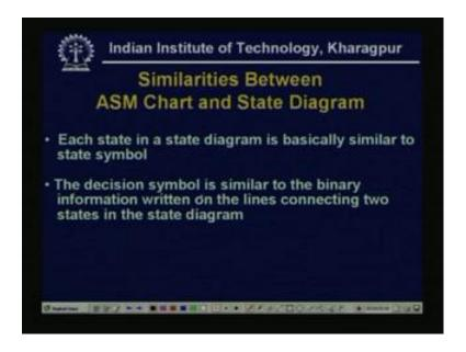
Now, what are the similarities between ASM chart and the state diagram, so each state in a state diagram is basically similar to state symbol, what we have seen the state symbol has also a name, just like our state diagram; a logical name is there. So, state in state
