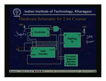
So, this is the hardware schematic for a 2 bit counter, just now what we have seen, see it has two parts, the controller part and the data processing part,
