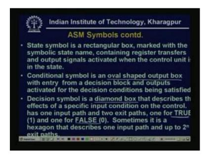
Now, state symbol is a rectangular box marked with the symbolic state name, containing register transfers and output signals activated, when the control unit is in the state. So, this is the rectangular type of box, normally it has some name and some binary coded value is given to the box. Second is the conditional symbol, normally this is a oval shaped output box with entry from a decision block and outputs activated from the decision conditions being satisfied.
