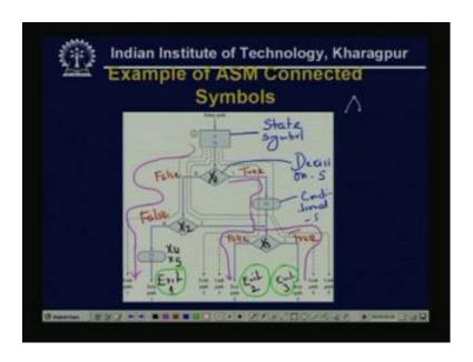
Now, this a simple example, that how the one ASM chart is can be constructed using the three type of symbols, so here we have taken one state symbols, I one entry point is here, so this is one state symbol. Now, this one is a decision symbol, this is a decision symbol, if it is false, if the decision symbols is written as a say X 1 the value. If it is false, then it is the entry point of another decision symbols say called X 2.
