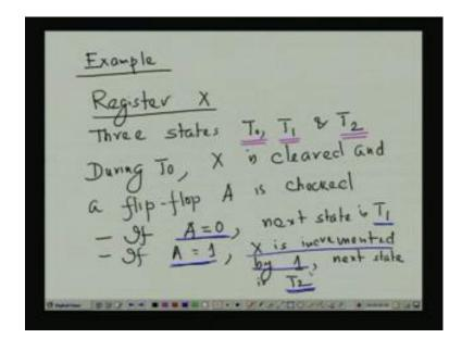
So, we take one example of an arbitrary ASM chart, say we are taking a symbol register X say we have a register X, there are three states T 0, T 1 and T 2. The machine is such of the synchronous sequential machine that we want to design. During that T 0, X is cleared and means it is reset or cleared or set to 0 and a flip flop A is checked.
