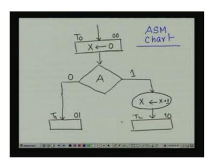
So, if we draw the ASM chart, first one state symbol and the register X is given, this is the states at T 0 as it is a state symbol, it has one entry point and one exit point. Now, it will go to a decision symbol and the decision symbol is A is checked, so the flip flop A is checked, the variable is placed inside the diamond box. Now, we know that diamond box has two exit point then, if A is 0; that means, if this is a false path, it should go to the state symbol T 1.
