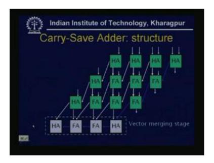
Now, using this carry save adder structure, some multiplier has been designed, where again that the first array is a set of half adders and the second array, third array and the fourth array is a set of half adders and full adders etcetera. So, this is carry save using carry save adder structure, where the last array is actually the vector, it is treated as a vector merging stage.
