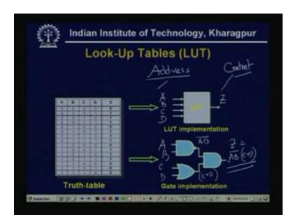
So, this is one example, as in the example I have shown there are one look-up table, it has four inputs A B C D and one output Z. See, this is the truth table, on the truth table this truth table is given the four inputs A B C D and this is one output. Now, see already we have using the Karnaugh map or many other strategies we have read, that we can derive the functions that what how that, what will be the Z, the output functions.
