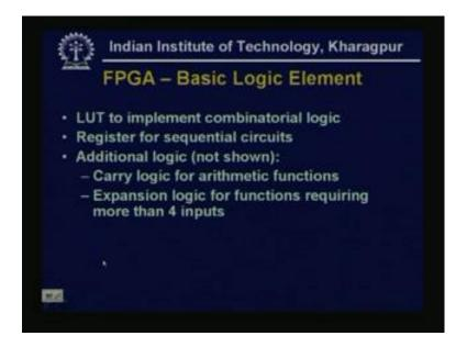
Now, how this FPGA basic logic element are implemented, as in the last class we have seen I mention that normally, look-up table is utilized or is the basic concept of a FPGA logic element. So, LUT to implement combinational logic, register for sequential circuits, additional logical and that this carry logic for a arithmetic function or expansion logic for functions requiring more than four inputs. These are the some common features of FPGA.
