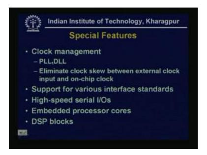
Now, there are some special features, say clock management normally the phase locked loop circuit or the direct link lock and these are being used for clock management which and this clock managements are needed to eliminate clock skew between external clock input and on-chip clocks. And the support various interface standards, high speed serial IO's, embedded processor cores and the DSP blocks, so mainly these are the special feature of FPGA.
