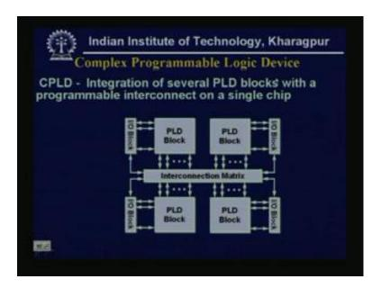
So, CPLD the complex programmable logic device, we can define as if, this is the integration of several PLD blocks with a programmable interconnect on a single chip. So, these are the PLD blocks and these PLD blocks can be any PLA, PAL or PROM type
