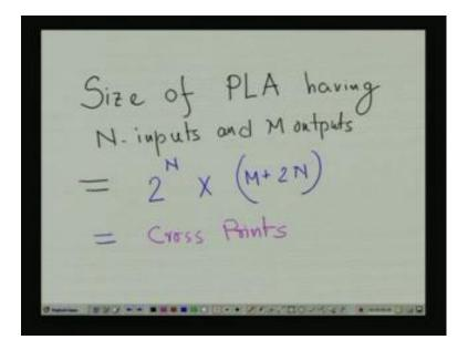
And that so, the size of PLA having N inputs and M outputs is equal to the power M by this is the number of rows, my M plus 2 N number of columns. So, this is a size, and so, these many number of cross points are also available, so these are my number of cross points, maximum number of cross points.
