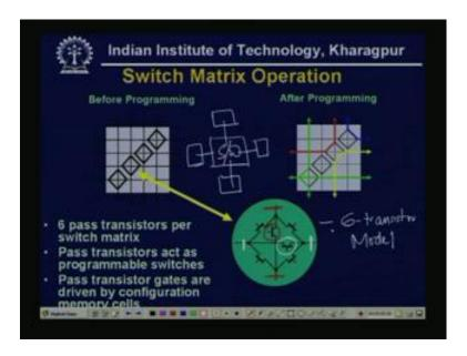
Now, if we with quickly see that switch matrix operations because, these are nothing, but a switch. See that, this is before programming as if the switches are kept and this is after programming means which one is connected to which line, as if this is, this line is see this red line means, this is one connection. So, this blue line, this is one connection like that, now this is actually, actual switching is we know that this is by pass transistors and these are act as a programmable switches.
