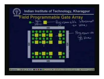
So, already this overall architecture we have once we have seen, now I describe one by one, so this is again a 2 D type of gate structures and if I consider these as a matrix. So, these as if, this small green one and the larger yellow blocks, these are the two types of matrix elements. And, the yellow one, we are telling this is my inter switch blocks or the programmable interconnection blocks, so this is my programmable interconnection blocks and this is my logic blocks.
