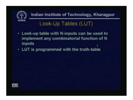
Now, look-up table is one of the important or this is the basic concept, so look-up table with N inputs can be used to implement any combinatorial function of N inputs. And look-up table is programmed with the truth table. So, we see that how the look-up table is implemented.
