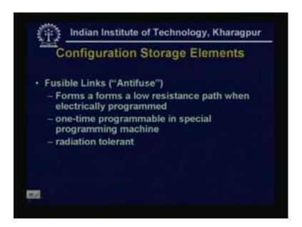
Now, configuration storage elements can be of fusible links, already we discussed that fuse or antifuse is use to gets the cross points on or off. So, it forms a low resistance path, when electrically programmed, now one time programmable in special programming machine and this is, this should be radiation tolerant.
