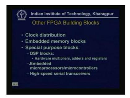
Now, there can be a other type of FPGA building blocks and they are for the clock distribution, the embedded memory blocks, special purpose blocks of DSP blocks, Hardware multipliers adders and registers, embedded microprocessors, micro controllers and high speed serial transceivers. So, clock distributions that, this is one circuitry and always these are needed, see if I have the, if we draw these things.
