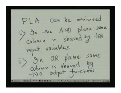
Say PLA can minimized, that number one that, in the OR plane or first we see the AND plane, in the AND plane same column is shared by two input variables. Or similarly in the OR plane same column is shared by two output variables, output functions two output functions, in this case, actually the PLA is partitioned row wise.
