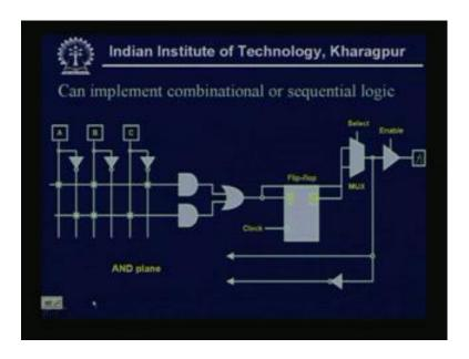
Now, not only combinational we have seen that sequential part also, can be realized by using this programmable and on the fixed type OR plane. So, any one of this, so far we have discussed the PROM, PLA, PAL, can be the PLD block.
