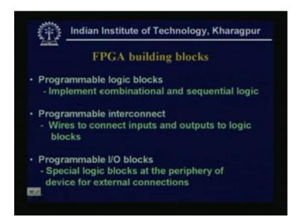
So, the FPGA building block, that it has some actually it has three types of blocks are available in the FPGA. The programmable logic blocks, which implement combinational and sequential logic, as already we have seen that PLD blocks can realize combinational as well as sequential blocks, now programmable interconnect. So, wires to connect inputs and outputs to logic blocks, just now we have seen.
