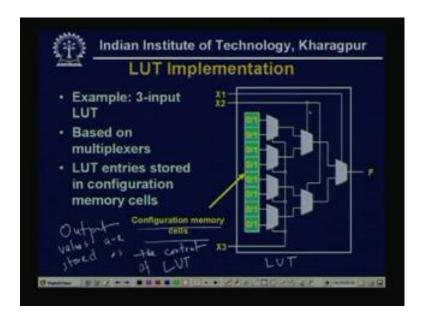
So, how it is implemented, see this is one multiplexer based, as if LUT entries stored in configuration memory cells and so, these are the contents of the memory. So, these are my, the output function the configuration memory cells means, as if output values are stored as the content of the table LUT and the three inputs X 1, X 2, X 3, they will be treated as the address of the memory.
