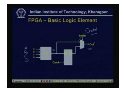
Now, this is one very simple or basic logic element, say I have one look-up table, see it has it has four inputs, the A B C D. So, the look there are four input variables A B C D are the inputs of the look-up table, see there is only one output, say one function F and that can be last as already we have seen and it or it can be selected. So, using this control line as the select this is my control from outside, when I want to take the output that can be chosen.
