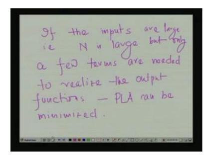
Now, as I already mentioned that, if the number of min terms, say if the input variable of the inputs are large means, that is N is large, but a, only a few min terms are needed to realize the output functions. Then, the PLA can be minimized and in this case the PLA is efficiently utilized, now another case is the, for PLA minimization.
