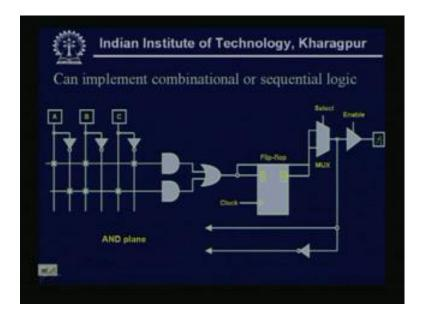
Now, some more advantages also there for this, fixed OR gate, OR plane, see earlier it was only combinational. Now, we can realize the sequential logic also by using a PAL structure, as this output plane, normally OR plane we call the output plane, because the output function is, can be computed or can, is taken from the OR plane. So, the, in the output of the OR, or the PAL plane PAL, we can add some d flip flop, so if we see this example.
