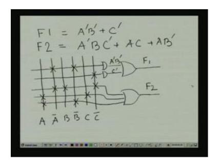
C dash AC plus AB dash and F 1 is A dash B dash plus C dash, so first we, how many, there are three inputs here A,B,C. So, if we draw the programmable OR plane, AND plane, so these are, there will be six, because six signal lines, because this is for A, this is A dash, this is B, B dash and C, C dash. So, this is A dash B dash plus C dash, so one cross will be here, one cross will be here, B dash, so this is, if I put one AND gate, that this is A dash B dash.
