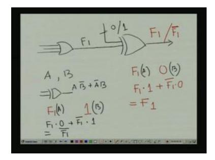
See, what we have done, now the, as if, the one we are considering, the output of this OR gate is a F 1 and that, we fed to the, one of the input of my EXOR, other input can be 0 or 1. Now, if we remember, if we remember the two input EXOR, see if A and B are the inputs of a two input EXOR, then the function will be AB bar plus A bar B, so here, if it is F 1 and 0 is in this line, F1,0. So, that means as if, this is my, see F 1, so this, as if this is my A and this is my A and this is my B.
