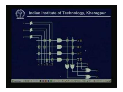
So, here, that OR plane gives me, that this functions, that F 1 and F 1 or F 1 complement and here F 2 or F 2 complement. So, this is my PLA design, a PLA design for a particular, next day we will be discussing that one, how the general structure of a PLA, that means, for N input M output equations, how the PLA can be designed. So, will continue, our this discussion in the next lecture
