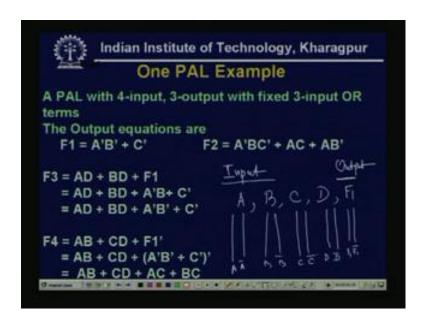
So, we can realize F 1, F 2, F 3, F 4 by using four input variable A, B, C, D as well as, the F 1 is again, as the one of the output function, F 1 as the F 1 and F 1 complement as the input variable. So, here the number of inputs are, the input variables are A, B, C, D and F 1, so that means, for A A bar, for B there are two lines B B bar, for C, C C bar for D, D D bar and for F 1, F 1 F 1 complement. And actually, they are coming from the, as the, these are, this is the output.
