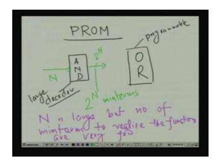
So, if you remember that, the PROM, if you remember, that in PROM that, this is a fixed AND array, it has, say it has N inputs and all 2 to the power N. So this output means actually, these are here, all 2 to the power N minterms can be realized and then it is fed to the OR plane, this is programmable. Now, see here it is N, N, any N, N can be very large, see if N is large, but number of minterms to realize the functions, are not so, so larger, they are small, they are few, are very few.
