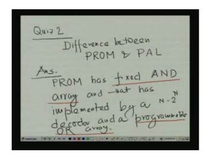
So, again quiz 2, answer is, the difference between PROM and PAL, so PROM, we have seen that, answer, the programmable ROM has fixed AND array and that has implemented by, a into 2 to the power N decoder and a programmable OR array. So, here the main thing is, it is a fixed AND array and a programmable OR array, whereas the PAL, it is totally different reverse or we can tell that, it is reverse.
