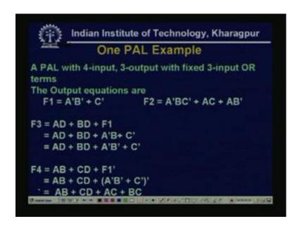
So, here, if we see one example, of another PAL example, that how we can realize this thing, say PAL with four input and three output, with fixed three input OR terms and output equations, there are four output equations, F 1 is A dash B dash plus C dash, F 2 is A dash B C dash plus AC plus AB dash, F 3 is AD plus BD, actually AD plus BD plus A dash B dash plus C dash. So, first we realize F 1, F 2 and then we will be seeing that F 3, F4.
