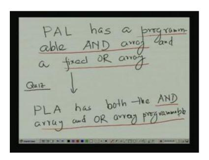
That, PAL has a programmable array logic, has a programmable AND array and a fixed OR array. So, this we can take it is total, totally reverse thing on the, if we consider the programmability. Now, question 3 was, the quiz 3, it was the difference between PAL and PLA, so already have seen, PAL has a programmable AND array and a fixed OR array. So, these will be as it is, it will be coming as PAL and PLA is, PLA has both the, has both the AND array and OR array programmable.
