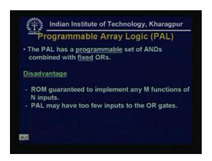
So, well, we have seen in details or we have read the details of PROM, now we see that, the actual architecture and the design of the PAL, the programmable array logic. Just now, we have seen the PAL has a programmable set of ANDs combined with OR, fixed ORs, that means AND array is programmable OR array is fixed. Now, what is the disadvantage, see, ROM guaranteed to implement any M functions of N inputs, because it has a fixed AND array and we have implemented that thing by a decoder.
