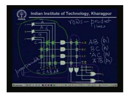
See, the PLA has both the AND plane and OR plane programmable, so this is my AND plane and this is the OR plane and both are programmable, so both are programmable. So, it has three inputs A, B, C and just like what we have seen that, both A and A bar are available that means, this is my A and this is A complement, B B complement, C C complement and that are given, we can write here also, this is C, C bar, B, B bar, A, A bar.
