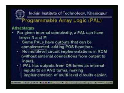
Now, what are the advantage, so given internal complexity, a PAL can have larger N and M, because it has AND fixed or OR fixed and AND programmable. So, it can handle, that larger input variables and as well as OR fixed, so as it is fixed. So, in that design itself, as it is a fixed OR plane. So, that M can be initially itself, that M can be the larger value can be selected, some PALs have outputs, that can be complemented adding POS functions, so this is a very important property.
