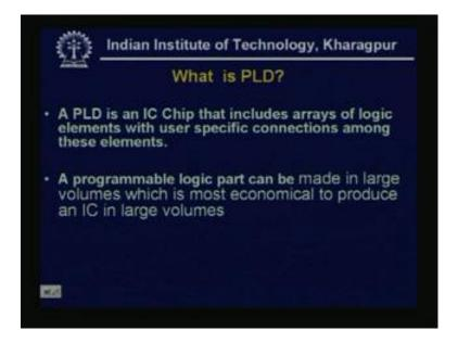
So, first we see, what do you mean by a programmable logic device or in short we call PLD. So a PLD is an IC chip, we think that includes arrays of logic elements, with user specific connections among these elements. Normally, it has two different arrays and they are, they can be programmed from outside. Now, we will see, how these arrays are programmed, what is the structure of this array, later and why it is so popular or what is the advantage.
