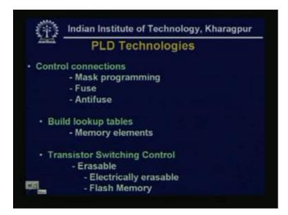
First, we see the control connections. So, these are, normally this mask programming or fuse and anti-fuse that are being used. We see that thing already, say if we, see like that...
