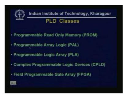
Now, we see what are the different configurations, normally we call the PLD classes. So these are programmable read only memory, PROM, programmable array logic, the PAL, programmable logic array, PLA, complex programmable logic devices, we call CPLD and field programmable gate array, FPGA. Now, one by one we will see that, what do we mean by all this classes, what are the differences etcetera.
