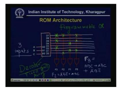
So, we see the design, see, if we draw, so this is my 3 by 8, so this is a nothing but a 3 by 8 decoder, it has 3 inputs, say A, B, C and there are 3 inputs. Now, there are, a 3 by 8 decoder, so 8 output lines 2, 3, 4, 5, 6, 7,8, there are 4 output lines. So, this is my, as if this decoder, this is the, this is the decoder, this give me the fixed AND gate, AND array,
