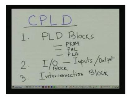
So, what we can tell, that CPLD, so if we take the CPLD blocks, so it has three components, one is that some PLD blocks that can be made by PROM by PAL by PLA. Second is the IO block, where the, from the inputs and outputs are fed or taken out, so this is IO block and then, the interconnection block, so interconnection block, that is between IO and interconnections or interconnection to PLD blocks. So, mainly these three are the, that the three basic blocks, that is there in the CPLD structure.
