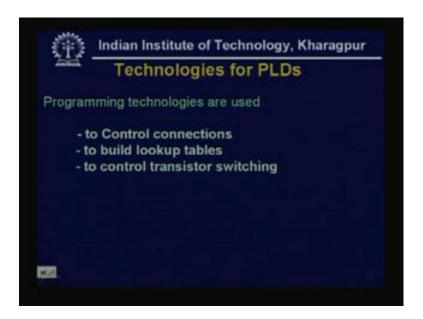
Now, what are the technologies for PLDs, technologies means, that mainly the programming technologies. Now, programming technologies are used to control connections, to build lookup tables and to control transistor switching, now one by one we see that thing.
