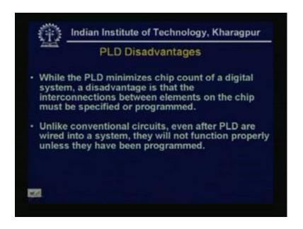
Now, what are the disadvantages, there are some minor disadvantages are there, because now the complex PLDs are used and while the min, PLD minimizes the chip count of a digital system, the disadvantage is that, the interconnections between elements on the chip must be specified or programmed. So, when that interconnections, this is once says it is a flexibility.
