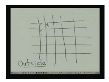
Say, as if, say this is some, some 2 D arrays, see this is some of the rows and say some of the columns are there, we will see later that how actually they are designed. Now, whether here there is a connection or not, that means, if I put a transistor here, say here or that can be in diode, that can be transistors, in this way if we put, then that can be programmed from outside. So, this is the user specification or depending on the requirement, what they want to design.
