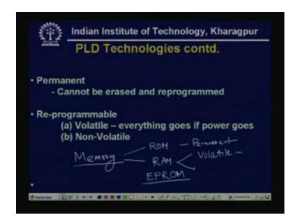
Then, normally PLD technologies are either it can be permanent, permanent means cannot be erased and reprogrammed. That means, the memory we will use if it is a ROM, read only memory type. We have seen that, if it is a lookup table base and lookup table can be implemented by memory and if this memory is a read only memory type, that means, it cannot be changed. Then it is permanent, cannot be erased and reprogrammed.
