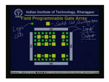
Now, another is field programmable gate array and nowadays, this is the, state of the art of the VLSI design. So, as I mentioned, that this PLD devices are one of the basic building blocks of the ICs now and as there large volume of design can be built or can be fabricated, on a piece of silicon. So, this field programmable gate array is nowadays an alternate to the normal CMOS ASIC. Now, we see the structure, this is similar to the CPLD.
