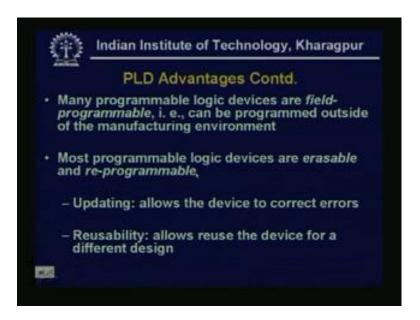
Now, some more advantages you see, that many programmable logic devices are field programmable, that is can be programmed outside of the manufacturing environment. Most programmable logic devices are erasable and re-programmable. This is one of the very important issue or the property, why the programmable logic devices are so popular or becomes the state of the art, of the digital design. See, they can be erasable and re-programmable.
