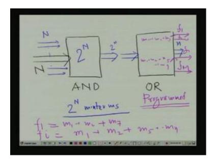
Say, I have 2 array, see this is my AND array, this is my OR array, say N input lines I am feeding N inputs, so as if, I am giving this in as, N variables, these I can represent as if, N, these are my N variables. So, here actually, 2 to the power N minterms, can be, this AND can represent 2 to the power N minterms, because N input variable, 2 to the power minterms. So if, these 2 to the power N minterms, output is actually 2 to the power N and that is fed to my OR array.
