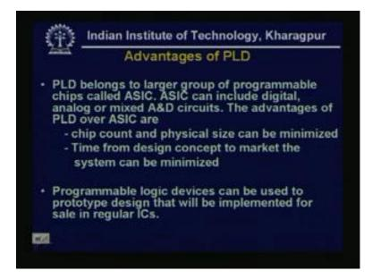
Now, what is the advantages of programmable logics, so PLD belongs to a larger groups of programmable chips called ASIC. So, we know that, ASIC is the application specific integrated circuit, we have, we discussed earlier and that can include the digital design, that can include the analog or mixed analog and digital circuits. Now, the advantages of this programmable logic over ASIC, means, if this is a pure digital analog or mixed type, where the program, PLDs are not there.
