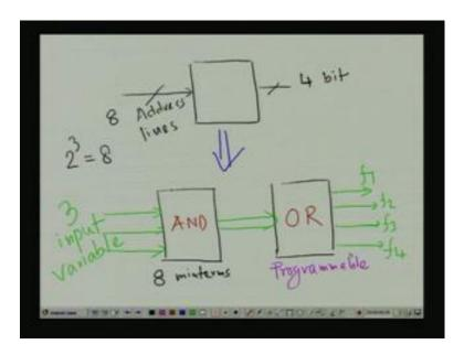
So, if we see one memory, it has 8 address lines and 4 bit content output. So, what we can do, if I want to get this thing by or I want to implement this thing by, PROM or programmable logic device, then this is my AND, this is my OR, so here 8 address lines. So, I need, I know 2 to the power 3 equal to 8, 2 to the power 3 equal to 8, so here AND gate, there will be 3 inputs, 3 input variable and number of minterms, that there will be 8
