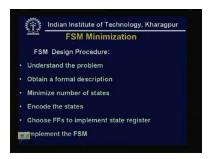
So, now what we have seen that last example, we have seen that, there are 7 states we have drawn, because it is a 3 input pattern should be recognized 0 1 0, that is why, we have given, the 7 states. Now, if we see the, full efficient design procedure, what we will be doing, first we should understand the problem, then a formal description, then minimize the number of states, because ultimately, our aim is to design and, or is to make a efficient design.
