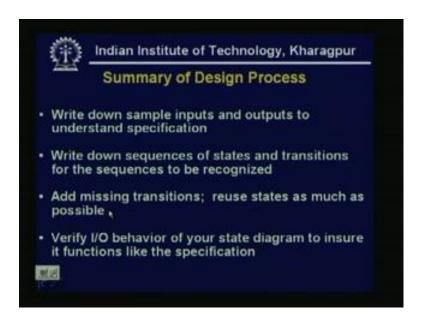
So, now if we summarize, the full design process, what we have done, first we write down, the sample inputs outputs, to understand the specification. Therefore, the pattern
