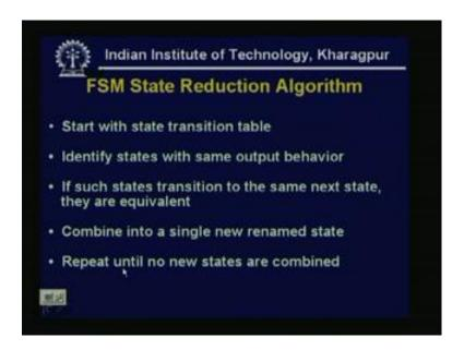
Now, there are several algorithms, exist for the state reduction, so what should be the algorithmic steps. So, if we start with state transition table, fist we already, we have defined for all possible inputs, what should be the output of the machine, then identify states, with same output behavior. So, first what we are doing, that the states we are identifying, which are giving the same output, now if such state transition to the same next state, they are equivalent.
