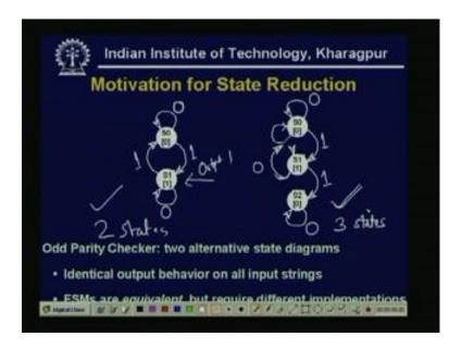
Again, we consider the, example the last day we discussed, the odd parity checker, so that means, one input pattern, if the number of 1's are odd, then it will give a 1 output, and otherwise it will be 0. So, there are, what we have seen there are two, alternative state diagram. See that, if, a initial state is S 0, then if 0, input as come any number of 0, means, it will be a even parity. Because no 1 is there, now if 1 comes, then actually, it will be a odd parity, giving output 1.
