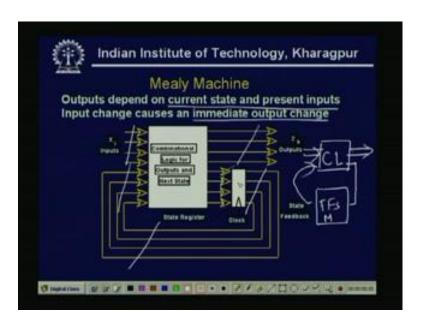
Now, if it is Mealy machine, the output depends on current state, as well as the present inputs. So, this is a difference, that for Mealy machine, that current state and present input, and the input change causes an immediate output change. That means the output change, occurs only when the input changes. So, what will be the general circuitry, that these are the present inputs, present outputs, and as these depends on the current states and present inputs.
