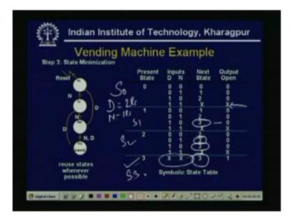
Now, first we see, the state table, so first is the what are the present state. So present states can be, that 0, 1, 2, 3 that means, S 0, S 1, S 2, S 0, S 1, S 2, S3 see, S 0, S 1, S 2, and S 3, only these are the intermediate states, from where the input, with 1 input, that 1 ticket can be delivered, and all are output state. So, if it is S 0 state, already we have seen, I can, I can give you 0 0 means, nothing as, been deposited, obviously, next state is 0, output is no output 0.
