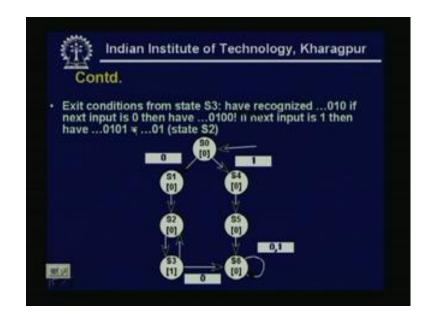
Now, exist condition from state S 3, so the exist condition from state S 3, have recognized that 0 1 0, if next input is 0, then have 0 1 0 occurs. Now, in next, input is 1, then have 0 1 0 1, so again that, what we have done, that we mainly we want to construct a pattern recognizer ((Refer Time: 56:42)) and the design principle, what the basic design approach ((Refer Time: 56:48)) what we have seen. That, first we have to realize the statement of specification.
