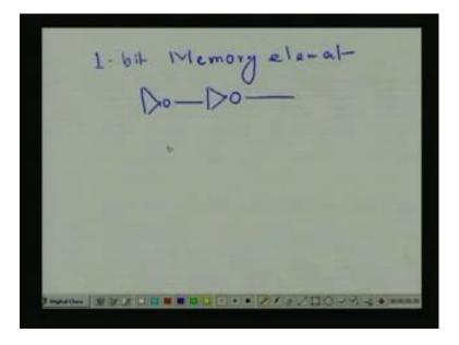
The one bit memory element that is by using inverter one NAND gate and if it is cascaded with another inverter that means, 1 NOT gate and another NOT gate.
