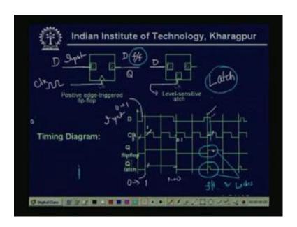
Now, again the D changes here the D changes at this position 0 to 1 the input changes input changes, but the clock here it is a level this is a 1 level, this is a 0 level. So, this is 1 this is 0 So, as it is a level sensitive, so the latch will it becomes 1, so the latch output becomes 0 to 1. Now, the similarly the D becomes slightly D becomes 1 to 0 slightly before the clock changes 0 to 1 see here also the clock level changes 0 to 1 level, so the first time that latch changes from 1 to 0.
