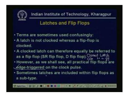
Now, we see that latches and flip flops, so these terms are sometimes used confusingly. So, we must clear this a the what is the difference between this two, see normally a latch is not clocked whereas, a flip flop is always clocked. So, initially when we have define the SR latch there was no clock only this is a two cross coupled NOR gate was connected. And S and R that 2 inputs are there, so a clock latch can therefore, equally be referred to as a flip flop, so S R flip flop, D flip flop.
