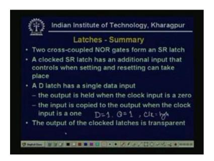
Now, so far we have discuss the latches, so if we summarize what we have read about the latches that two cross coupled NOR gates form an S R latch the set and reset latch. A clocked S R latch has an additional input that controls when setting and resetting can be taking place. A D latch has a single data input the output is held when the clock input is 0, the input is copied to the output when the clock input is in 1. Because we have seen
