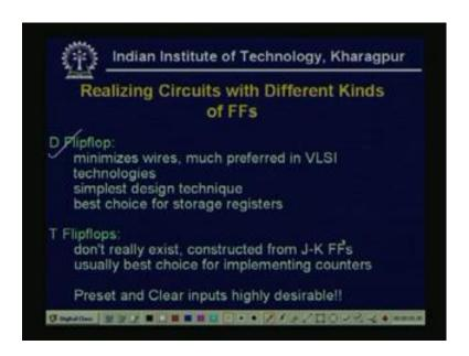
Now, the simple D flip flop, so it minimizes wire because we have seen that it is it is a simplest kind much preferred in VLSI technologies. Because it is very efficient and takes very less hardware simplest design technique and best choice for storage registers. That means, for one bit storage this is the number 1 the D flip flop. Normally, T flip flops do not really exist this is the, same flip flops means a toggle type of flip flops and, but
