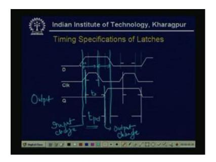
Now, if we consider the latch, If we consider the latch then similarly that this is again D and clock if we give that, so this is a clock latch. Then, similarly, the here the D changes from 0 to ,1 the clock changes from 0 to 1 this is the position. Here the clock changes from 1 to 0 and here the D changes from 1 to 0. Now, similarly that when D changes from 0 to 1 here the Q changes that means, my output the output changes from 0 to 1 is this position.
