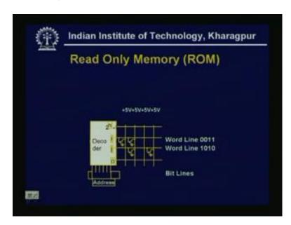
But before that, we see that how the memory structure is so normally this is a read only memory. See that here, there are some decoder lines where the decoder input are the memory addresses. That means, say if we if we write in this way.
