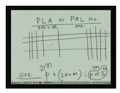
Whereas that for PLA or PAL, that is for PLA or PAL size that this size that input lines are these are 2 n, where for any n variables this is m outputs. So, this is 2 n plus m 2 n plus m columns and rows will be the only the P number of terms, where this P is very very less than the 2 to the power n.
