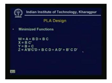
Now, if we realize or if we minimize the functions then we will get the solution as. Now, if we realize or if we minimize the functions then we will get the solution as the W is A plus BD plus BC by minimizing the Karno maps, X is BC dash Y is B plus C, because we will be getting here.
