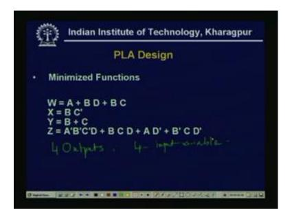
Now similarly, the Z will be getting that A bar B bar C bar D plus BCD plus AD bar plus B bar CD bar. Now, if we mainly that this is now will becomes a very simple function that there are four outputs. So, there are four outputs this A B C D, four input variable functions.
