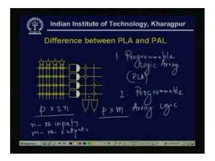
Now, we have two different type of programmable array logic 1 is called the programmable logic array, programmable array logic or PLA and another is programmable. Now, what is the difference between two, so far we have discussed, where both the AND planes and OR planes can be programmed. Tat means given some n input lines or 12 number of columns in the AND gate and say the different product terms can be P, then the AND plane size is AND plane size is P by P by 2 n.
