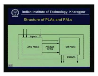
Now today, we will see that the logic design with PLA's, Last time, we have seen that mainly the programmable arrays or programmable array logics can be constructed by defining two planes the AND plane OR plane. The AND plane generates the all the product terms and the product terms are fed to the OR plane, OR plane generates the output.
