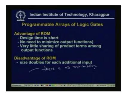
Now, the programmable arrays of logic gates, see that advantage of ROM is that design time is short and no need to minimize output functions. It is a very little sharing of product terms among output functions. See here, that actually all the min terms or all the products terms are exist, so there is no need to minimize the output function.
