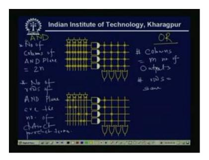
This is the overall structure of AND plane and OR plane, that particular example this should be the realization. Now, what we are discussing that alternative representation of the AND plane and the OR plane. See here that AND plane, if is a n variable input, what we have seen, that if it a n variable input, then the number of columns of AND plane number of columns of AND plane equal to 2 n.
