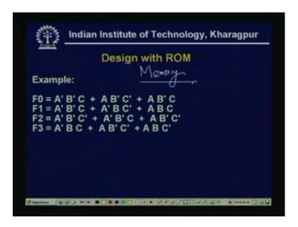
So, we will see that, how memory can be used as the logic design. Again here we have seen, we have taken three variable examples having four output expression of it and we will see how this can be designed using a memory.
