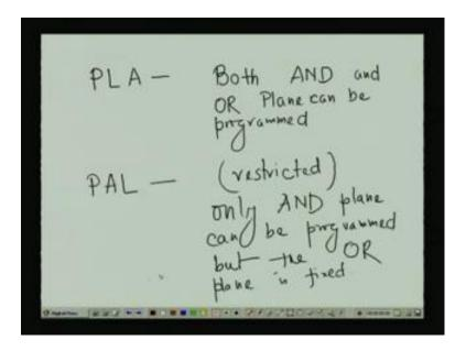
PLA, both AND and OR plane can be programmed whereas for PAL it is a restricted design or restricted with respect to the PLA mean only AND plane can be programmed, but the OR plane is fixed. So, this is one this type of structure.
