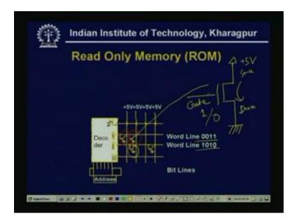
See here, these are the addresses and if it is n address lines, then this will be a 0 to 2 the power n minus 1 that many number of output lines. Now, this output lines they are called as word line, they are see here this is a word line 0 0 1 1 means that here, this is will be treated as 0, this will be treated as 0 or 0 0 1 1. So, this will be actually this column lines they are connected to 5 volt supply all are connected to 5 volt supply.
