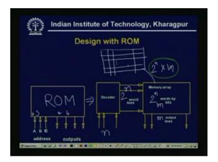
Now in this way, we can define that the ROM structure, now how this ROM can be used for the designing circuit, say this is my ROM with three inputs and four outputs. Now, this can be first this can be realized as if it is a decoder. So, decoder input is n the number of word lines are 2 to the power n and this is a 2 to the power n words by m that many number of bits if it is has m output lines. So, if we see actually here, there are 2 to the power n by m that many number of words are there.
