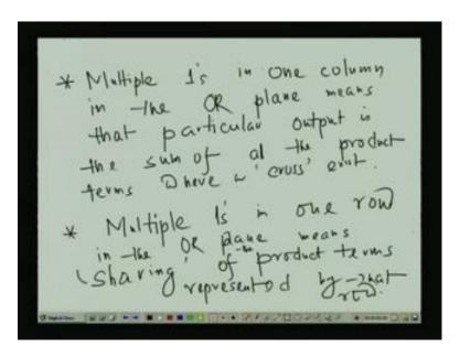
So, what we are we have discussed in the last class also, that the multiple ones in the or in one column in the OR plane means that particular output is the sum of all the product term, where a cross exist. But, multiple ones in one row in the OR plane means; that means, the sharing of that product terms represented by that row.
