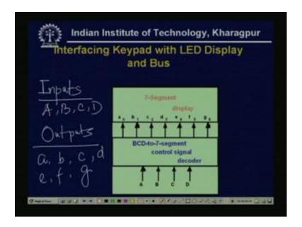
So, overall thing this is a BCD to seven segment control signal decoder. Say here, I want that this ABCD are my inputs. So this is a problem or this is combinational circuit design where the inputs are A B C D and outputs are that the seven segments a b c d, a b c d e f g the seven segments. So, this is a BCD to seven segment control signal decoder, we can represent this problem like that
