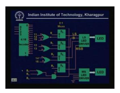
Now, using decoder and multiplexer I can design the circuits, this is my overall design say I have used a 4 to 16 decoder. So, these are my a b c d lines these are my four inputs and I have used 4 2 to 1 multiplexer which are actually driving the least significant LED driver and the most significant LED driver is a 4 bits and accordingly the LED are displayed. That means that particular segments of the LED are selected and they are displaced. So, this is the overall circuitry
