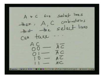
AC should take that say, if it is AC are the select lines. So, if A and C are select lines. Then the combinations AC can take, AC combinations that the select lines can take or we can think this as the control inputs are 0 0 0 1 1 0 1 1. See 0 0 means A complement C complement this is A complement C 1 0 means A C complement 1 1 means AC.
