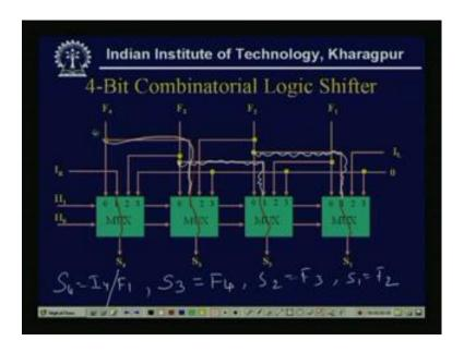
Now, first we see the normal combinational logic shifter see this is 4 4 to 1 multiplexer we have used. This is my MUX 1 MUX 2 MUX 3 MUX 4 or reversely we can take that outputs are S 1 is to S 3 S 4, and the functions that F 1 F 2 F 3 F 4 that we want to implement or we want pass that the as the output.
