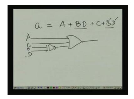
If I consider a equal to A plus BD plus C plus B complement D complement, see if it is not a AND OR gate any using any other logic gates, if I want to minimize the gates. And say, I have all are different type of gates are available I have that option that AND OR XOR XNOR whatever that all possible gates that are available, it is not a AND OR realization.
