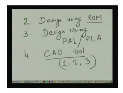
Now, the second can style can be that this can be a design using the ROM, so far we have not read the memory design using the read only memory we can also design this thing. This can be design using some programmable array logic it is called PAL or PLA programmable logic array or some CAD tool if it is a big design even some CAD tool can also synthesize or realize this function in different way.
