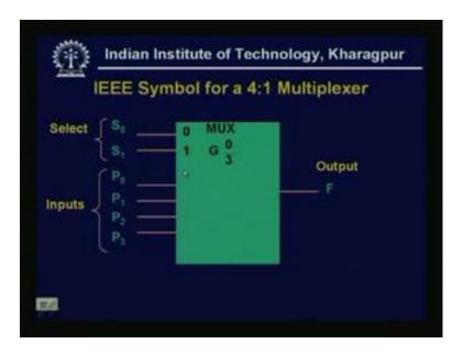
So, answer is, see that already we have discussed the 4 2 1 multiplexer design it has 2 select lines. And, 4 input lines 1 output lines and this is the algebraic symbol for 4 to 1 multiplexer, we will use this multiplexer to design a shifter 4 bit shifter.
