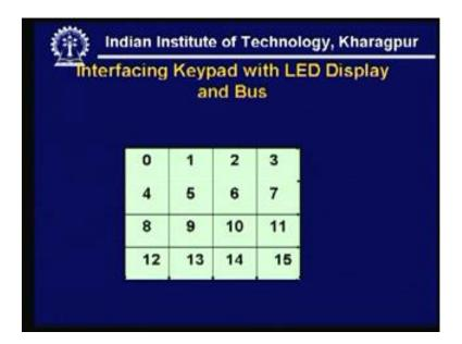
Now, our problem was our design problem was the interfacing keypad with LED display and bus. So, see if this is my keypad say I have 15 such keyboard I want that when I press 1 key day that number 5 key then that binary should be that should be or in that display board that five will be activated. And for that, I have to for that is that particular segments of the seven segment display must be selected.
