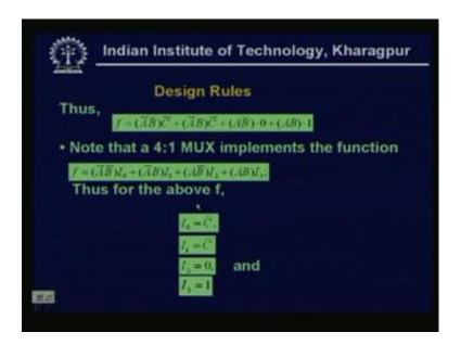
So, already we have seen this is my function. If we want to realize that using multiplexer that 4 to 1 multiplexer implementation because, there are 2 I have selected 2 control lines or select lines. And so for 2 control lines there will be 4 inputs, 4 primary inputs they C bar, C bar 0 1.
