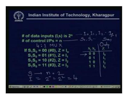
So, in general what we can tell that number of data inputs is 2 to the power n and number of control input is n, control input means my our select lines. So, this is my select lines should be S 0, S 1 up to S n, then my number of data inputs is I 0, I 1, I 2 then I 2 to the power n minus 1. So, here actually S should be n such lines, so it will be S 0 to S n minus 1 and for that n values it will be input should be 2 to the power n number of inputs, means 0 2 to the power n minus 1.
