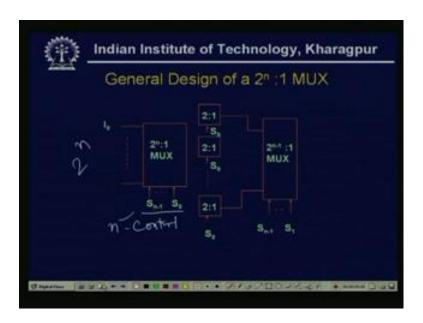
So, if we see that general design... Now if we generalize this design structure... So generalize I have n control lines, n control inputs then 2 to the power n primary inputs. It is fed to a 2 to the power n to 1 multiplexer. How I can design that thing in a hierarchical structure? So, 2 to the power n, so I need that n number of or 2 to the power n minus 1 number of 2 to 1 multiplexer.
