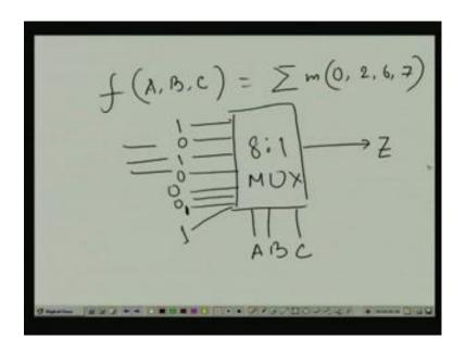
So, this combinational circuits what we can tell that the combinational circuit that a 3 variable combinational circuits f A, B, C is sum of m min terms are 0, 2, 6, 7. That is nothing but, a 8 to 1 multiplexers, where these values are A, B, C 3 select lines and the output will be only this 0, 2, 6, 7 lines. In these inputs are, 1. That means, this is 0, this is 1, 3 line is 0, 4 line is 0, 5 line is 0, 6 line is 1 and 7'th line is 1. So, this is the realization using multiplexer.
