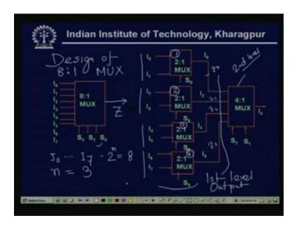
Now, if I apply the same thing for constructing a 8 to 1 multiplexer, so we can write that design of 8 to 1 MUX. Now, for 8 to 1 MUX there are 8 inputs, primary inputs are 8 that is I 0 to I 7. So, my 2 to the power n equal to 8, so n equal to 3, so I need 3 control inputs. So, in this way I define my or I choose how many control lines will be there or how many select lines will be there, so 8 inputs I 0 to I 7 and there are three select lines.
