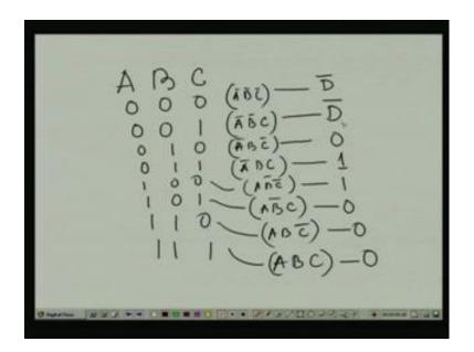
See, now I write the 3 select lines A B C these are 0 0 0, 0 0 1, 0 1 0, 0 1 1, 1 0 0, 1 0 1, 1 1 0, 1 1 1. What are the terms, see this is my A bar B bar C bar, this is my A bar B bar C, this is my A bar B C bar, A bar B C, A B bar C bar, this my A B bar C, this is my A B C bar and this is my A B C. ((Refer Time: 52:19)) Now, I see which are there for A bar B bar C bar D bar is there and for A bar B bar C D bar. So, for this 2 it is C C bar this is D bar, so for this my output should be D bar.
