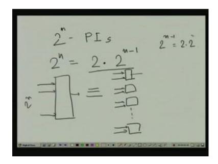
Why, see I have 2 to the power n primary inputs now 2 to the power n can be written as 2 into 2 to the power n minus 1. So, instead of applying 2 to the power n to the at a time the primary inputs these are 2 to the power n what I can do? These I can replace by say 2 to the power n minus 1 number of 2 to 1 multiplexer, where every multiplexer has 2 inputs, so this will be 2 into 2 to the power n minus 1.
