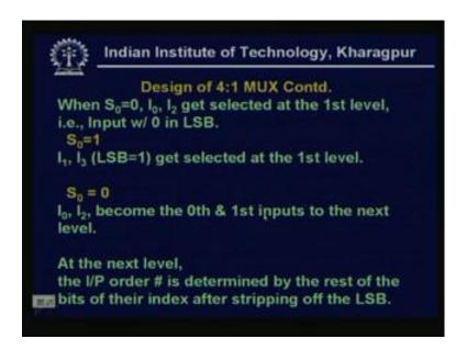
So, when S 0 is 0, I 0 I 2 get selected in the first level and when S 0 is 1, then I 1 I 3 get selected at the first level. So, if S 0 equal to 0 this become the 0'th I 0, I 2 0th and the first inputs to the next level. Now, at the next level mean the second level the input, output determine by the rest of the bits of their index after stripping off the LSB.
