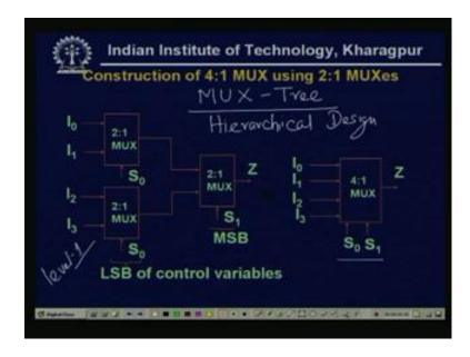
Now, that 4 to 1 multiplexer using 2 to 1 multiplexer, we call this is as a MUX tree or multiplexer tree, this is in general called the MUX tree or sometimes it is called the hierarchical design of MUX's, this is the hierarchical design. So, we take 2 to 1
