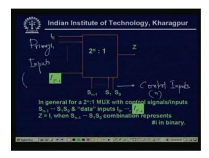
Now, today we will see first the general structure, so if now we draw the general diagram, then this will be my n control inputs these are my control inputs and these are my primary inputs. So, for S 0 to S n minus 1 means n control inputs primary input should be 2 to the power n and only 1 output.
