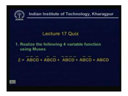
So, we take that the quiz question for this lecture, that realize the following 4 variable function using multiplexers and the function is Z is A bar B bar C D bar plus A B bar C D bar plus A B bar C D bar plus A B C D. So, today what we have discussed the design procedure, the design rule using that we can design this thing, so we will end the today's lecture here.
